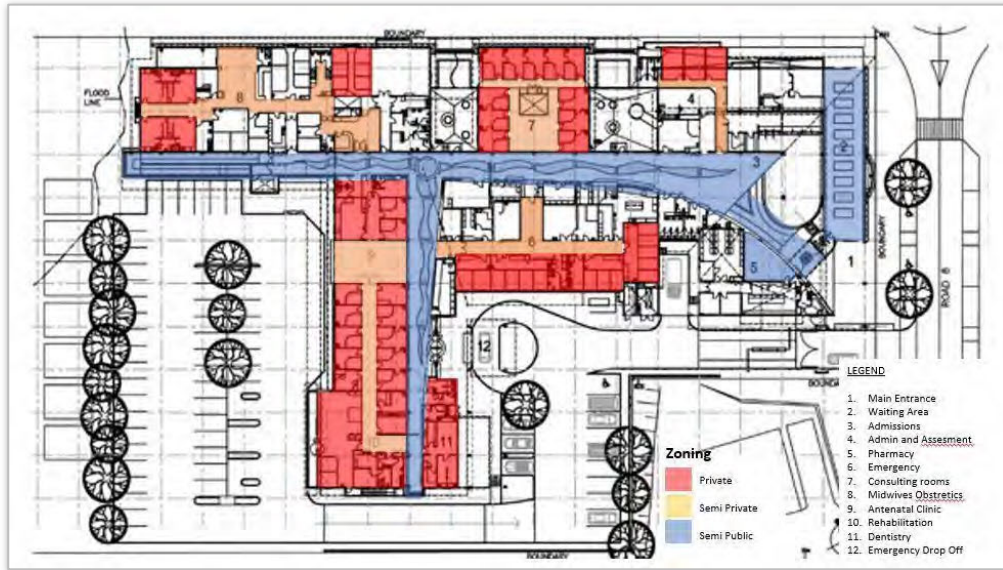
Figure 68: Floor plan highlighting the privacy gradient (Source: https://www.zaiconsultants.co.za/umkhumbane.htm : [accessed 07-11-2023] adapted by author)
