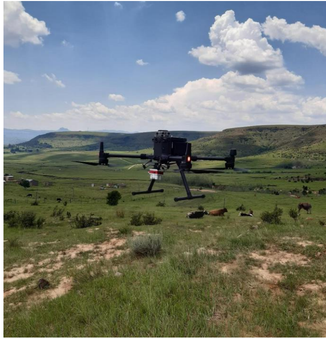
Plate 6.1: UAV mid-flight prior to autonomously flying its designated path to capture images, Okhombe Valley, KwaZulu-Natal Drakensberg, South Africa
