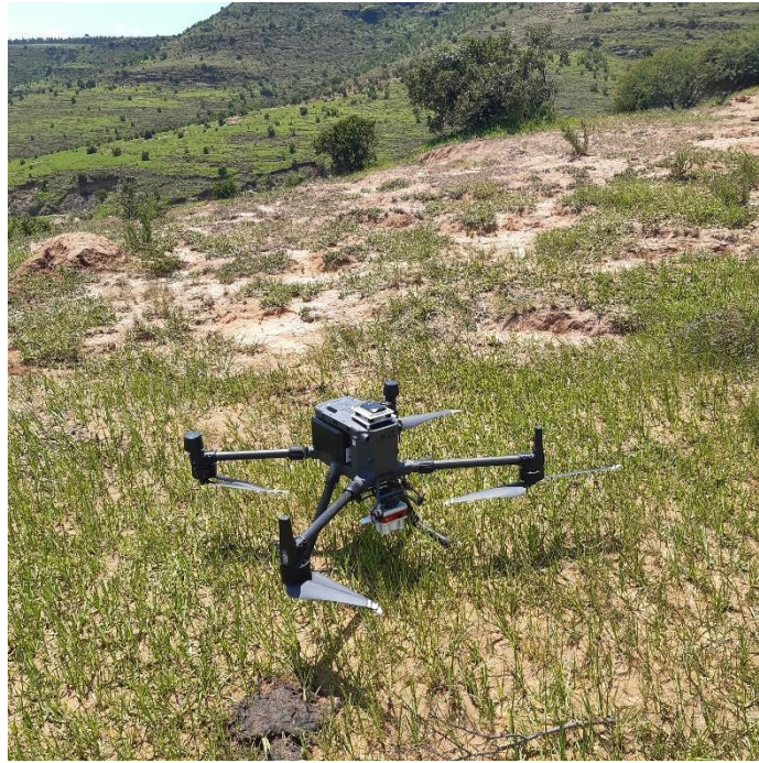
Plate 2.1: The Micasense Altum Multi-Spectral and Thermal imagery device on a UAV.
