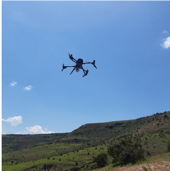
Plate 4.1: The UAV used to autonomously fly above the gully site (Okhombe Valley, KwaZulu-Natal Drakensberg) to capture images to determine plant health and map erosion, image taken with UAV at 5m height above the ground.
