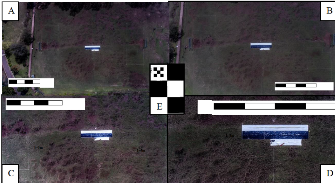
Plate 1: The pilot study images from the UAV at different heights focussing on a test pattern sheet for measuring pixel density, to determine the pixel density of each image at each height. An at a height of 100m, B at a height of 75m, C at a height of 50m, D at a height of 25m and E image of the PDRC. Scale is dependent on the height at which each image is taken and is shown in the corner of each image.
