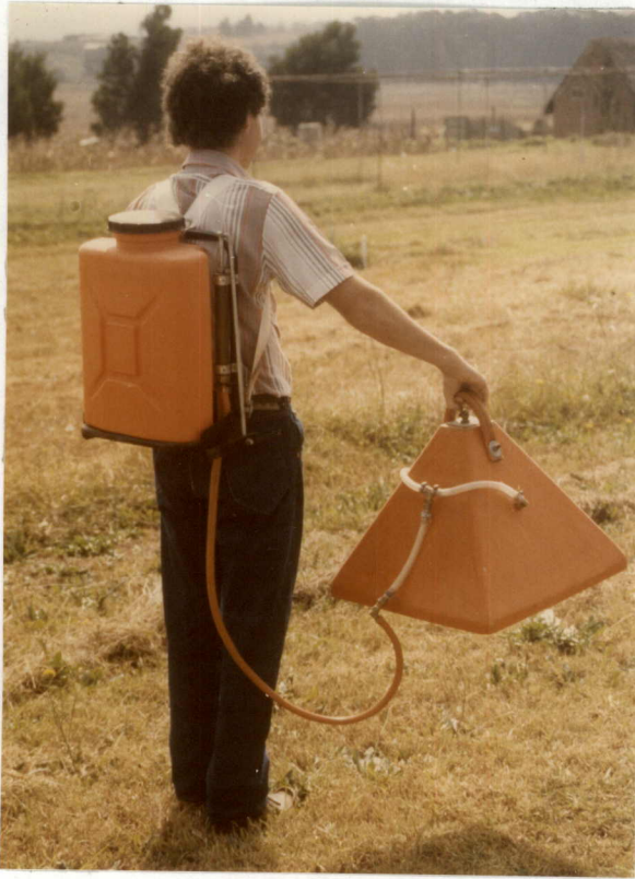
Plate 6A The knapsack and shield used in the directed-spray trial. X 0,4.
