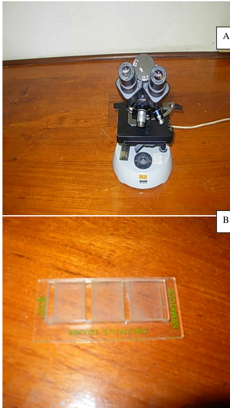
A. A Microscope used in the lab analysis B. Mc Master Slide
