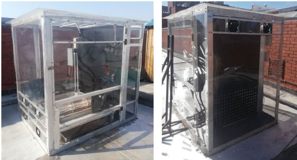
Figure 3-1: Greenhouse Solar Thermal Dryer –front/side of the greenhouse (left) and back/side of the greenhouse (right).
