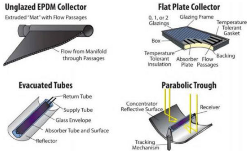
Figure 2-12: Examples of some of the solar thermal technologies.
