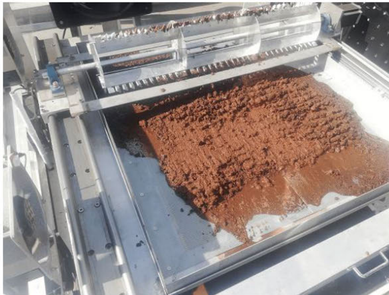
Figure 3-9: Wet soil test with 15 kg soil at 70 % moisture content.
