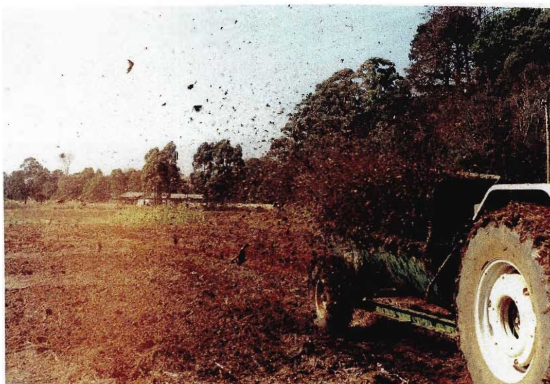
Figure B Fresh sludge being applied using the muck spreader. Much of the material is deposited in a 3m wide band adjacent to the path of the vehicle.
