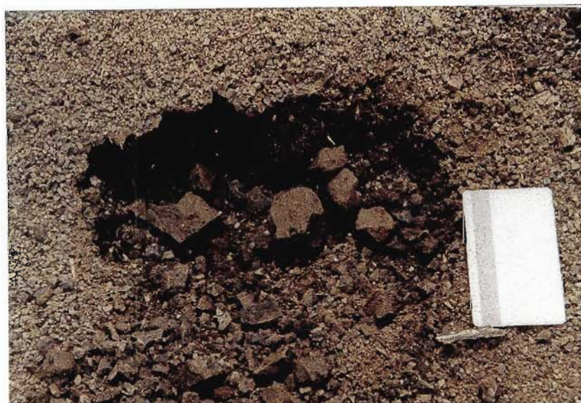
Figure 8.10 The breakdown of WTS aggregates showing the much finer grade of material at the plot surface. Below a few centimetres the material is much coarser in grade.
