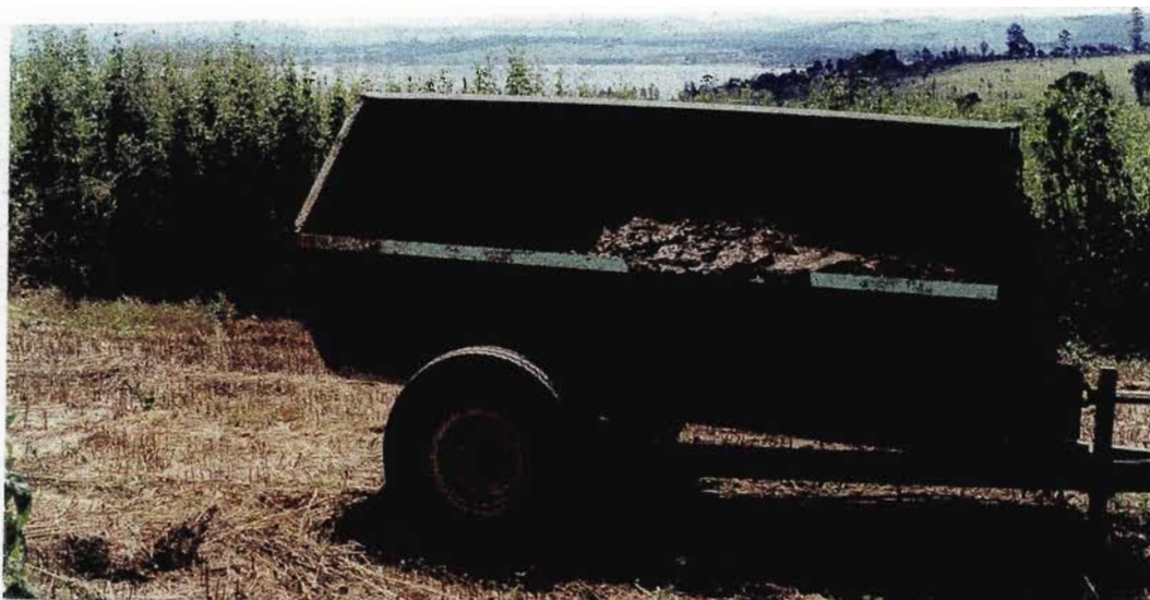
Figure A The muck spreader that could be used for the disposal of fresh sludge.
