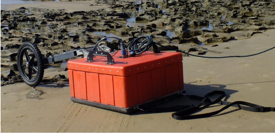
Figure A.1. 200 HS Antenna used to collect GPR data.
