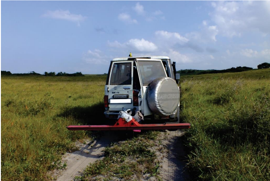
Figure A.3. Image of Cobra plug-in ground probing radar antenna (SUBECHO 40) mounted onto the back of a vehicle and transported along dirt road to collect data.
