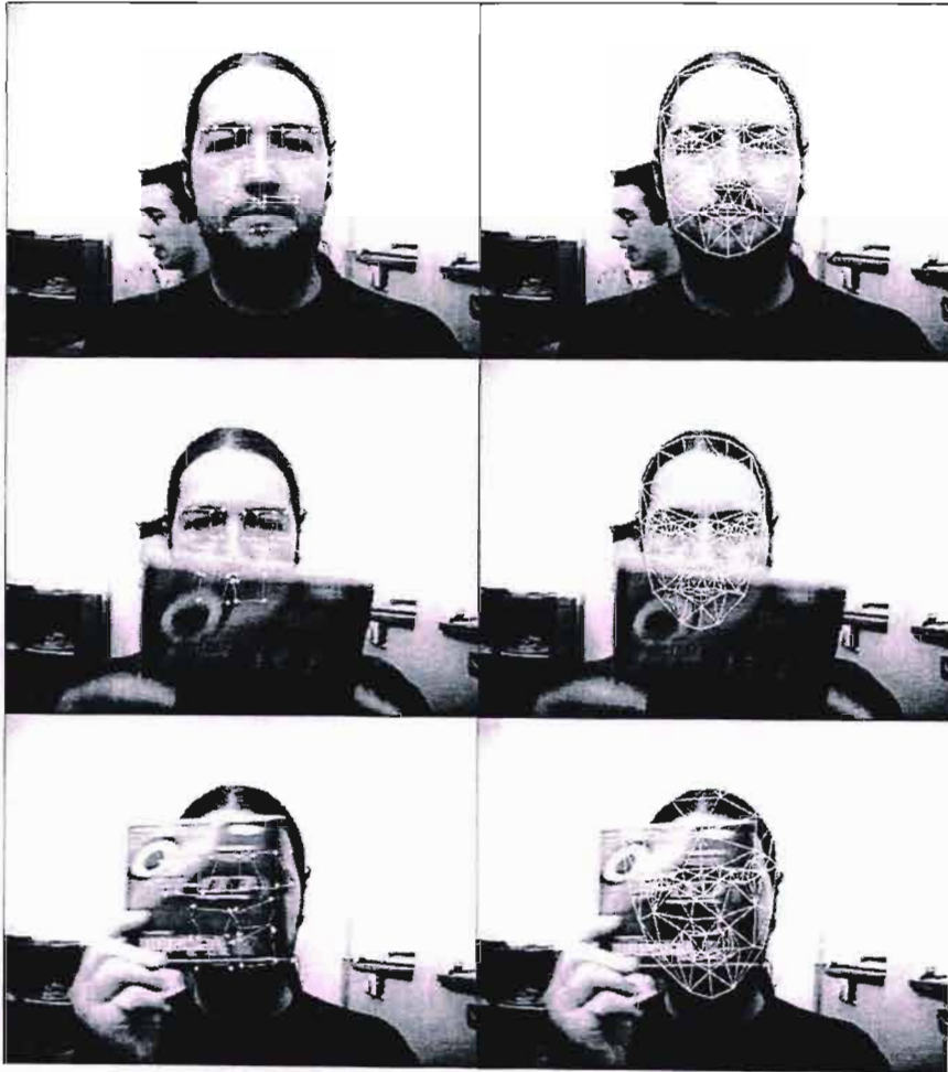
Figure 6.14: Tracking failure due to full occlusion.
