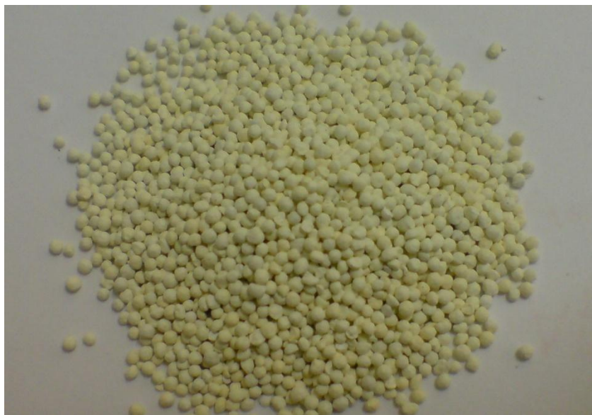
Figure 9.3: Photograph of 1 mm diameter sorbent after reaction with 4.15 mole % H 2 S in N 2 at 540 °C. Note the pale yellow colour with no carbon deposits.
