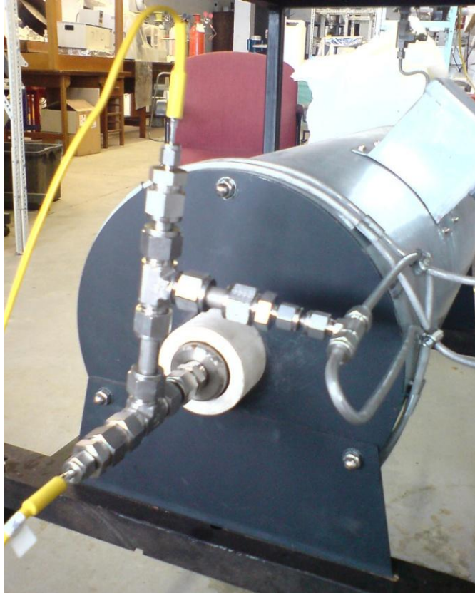
Figure 7.11: Photograph of gasifier furnace. The inlet thermocouples and vapour mixing point are clearly seen. The pipes have also been wrapped around the furnace to vaporize the liquid fuel. This was before insulation was added.
