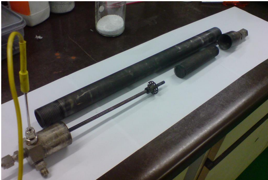
Figure 7.13: Photograph of the desulphurization reactor. The inlet thermocouple is still attached. The support grid is in the centre of the tube, secured on the thermocouple. The spacer maintains the integrity of the sorbent bed. The reactor tube was threaded to allow the sockets to be screwed on.
