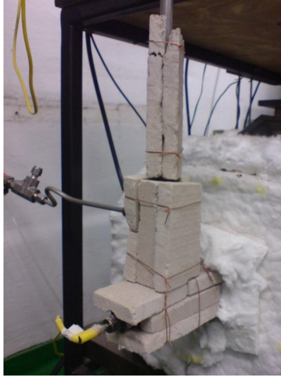
Figure 7.12: Photograph of the outlet of the gasifier. Insulation board was used for insulation. The thermocouple is visible, as is the pressure relief valve. The gas travelled up the pipe to the desulphurization reactor.
