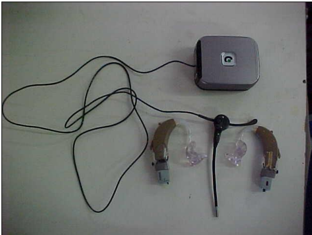
Figure 69. Campus S transmitter and receivers.
