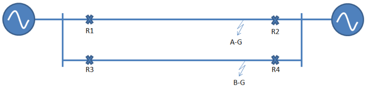
Figure 2.25: Illustration of a cross country fault
