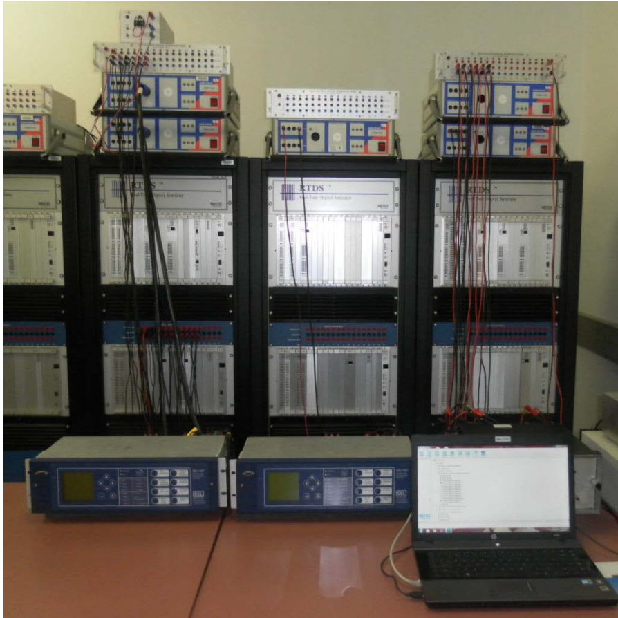
Figure 4.8: Hardware-in-loop connections between the SEL 421 relays and the RTDS simulator used for the research
