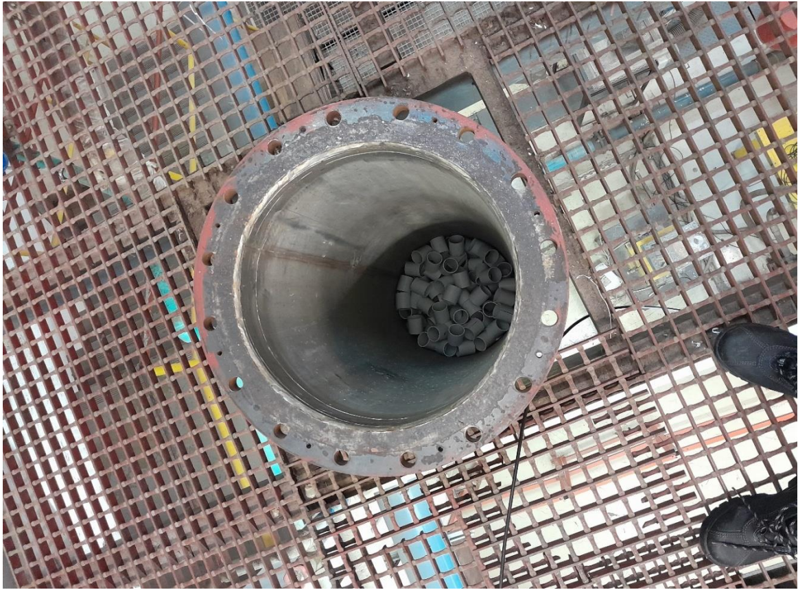
Figure 3-15: Uniform Packing Arrangement
