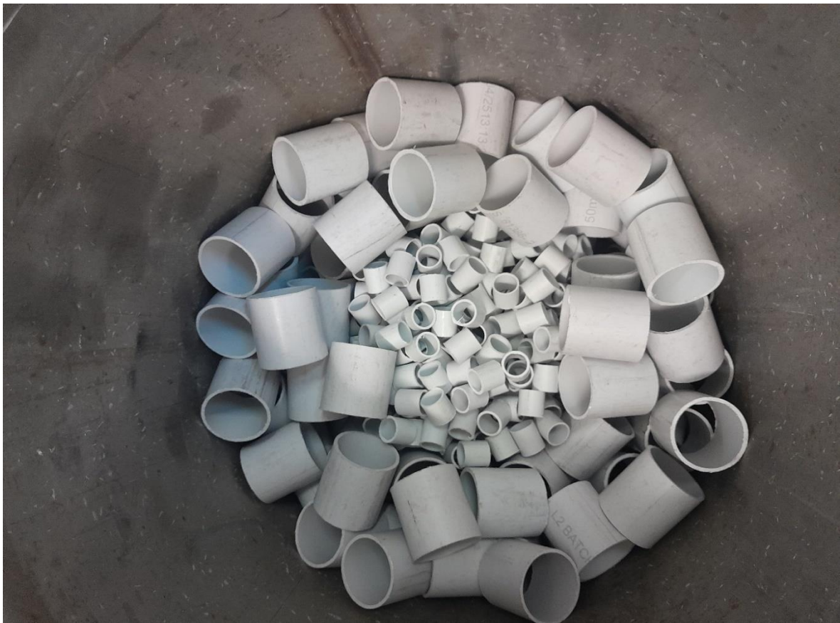
Figure 3-18: Non-Uniform Packing Arrangement (Small packing at the center)
