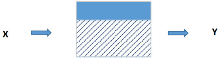
Figure 4-2: Non-Uniform Packed Bed (small packing at the wall side)
