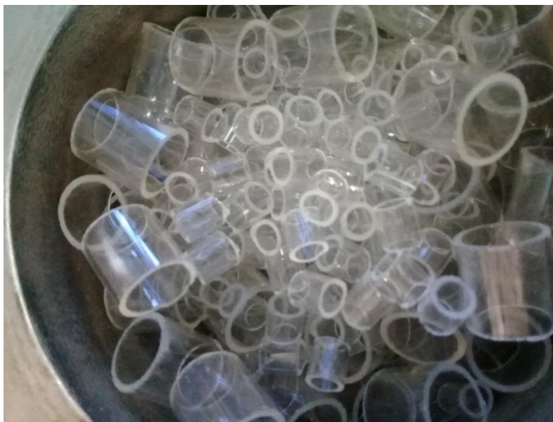
Figure 3-10: Non-Uniform Packing Arrangement (Small packing at middle (midway between center and side))-
