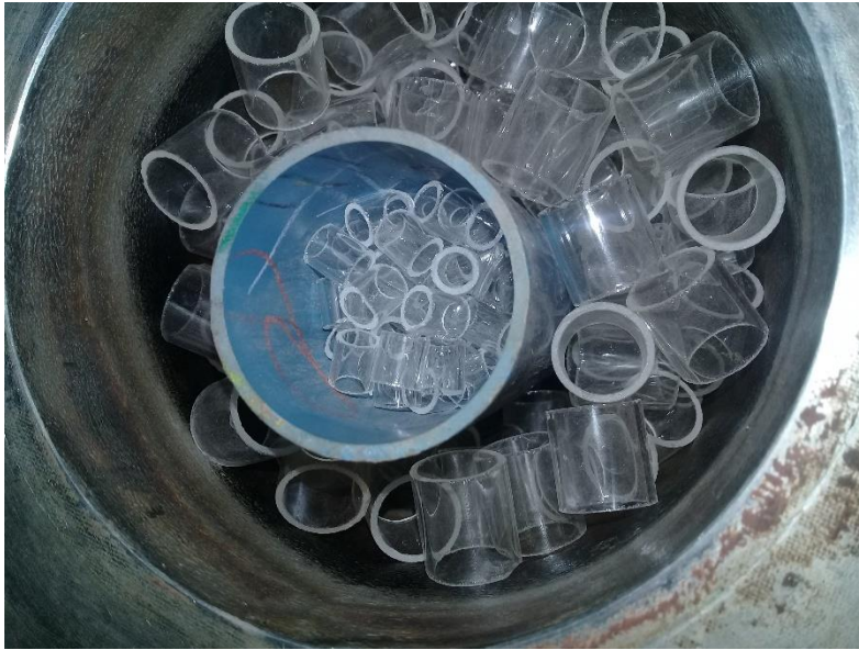
Figure 3-9: Non-Uniform Packing Arrangement (Small packing at middle (midway between center and side))-
