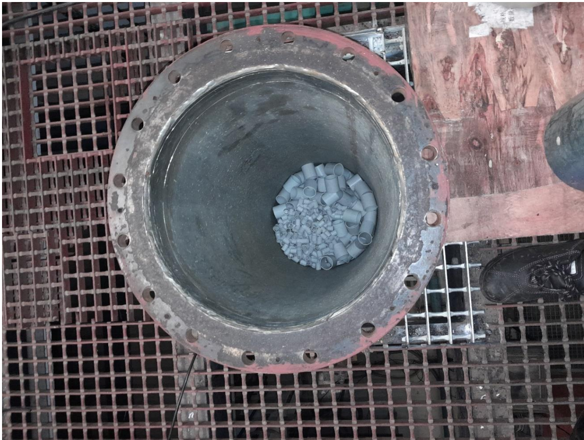
Figure 3-17: Non-Uniform Packing Arrangement (Small packing at the side)- During Experiments
