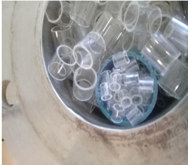
Figure 3-5: Non-Uniform Packing Arrangement (Small packing at the side)- Loading Process
