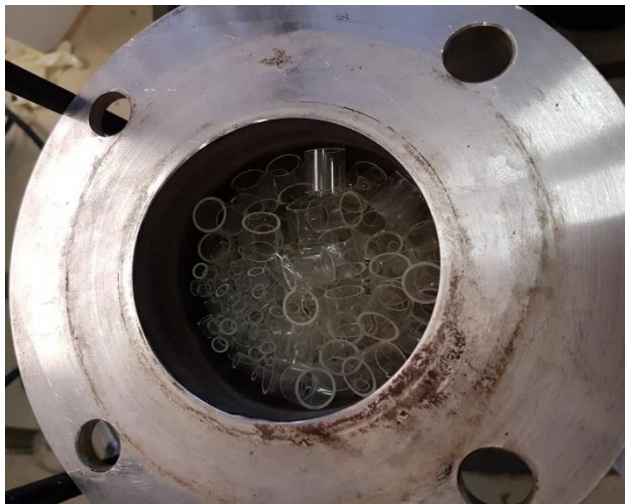
Figure 3-6: Non-Uniform Packing Arrangement (Small packing at the side)- During Experiments
