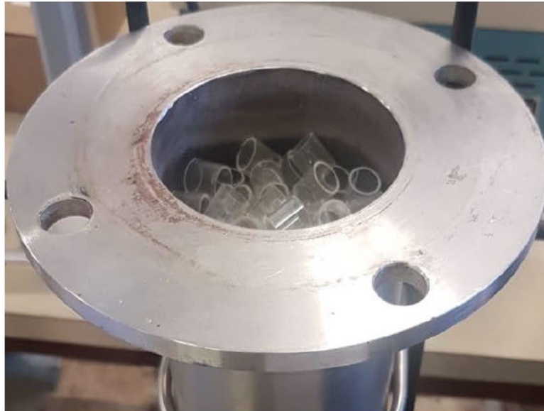
Figure 3-4: Uniform Packing Arrangement
