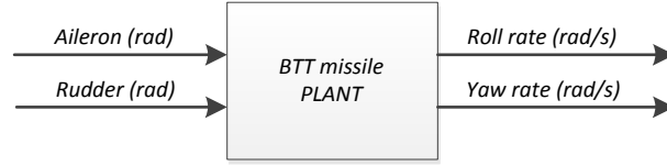
Figure 3.1.2 Plant input and output variables
