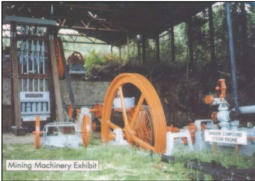
Plate 13.4. An exhibit of the Tandem Compound Steam Engine that was used at Millwood in the southern Cape (Duff, 2004).
