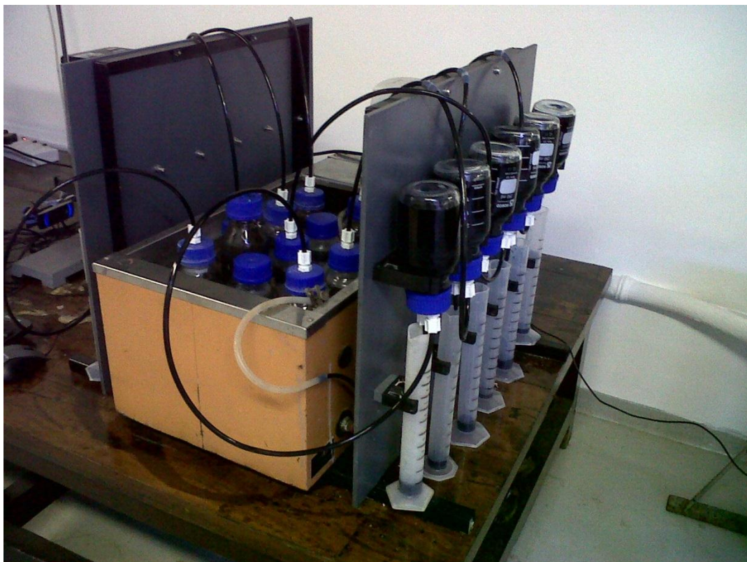
Figure 4.16: Photograph of showing the attachment of the serum bottles in the water bath to the inverted bottles filled with sodium hydroxide solution
