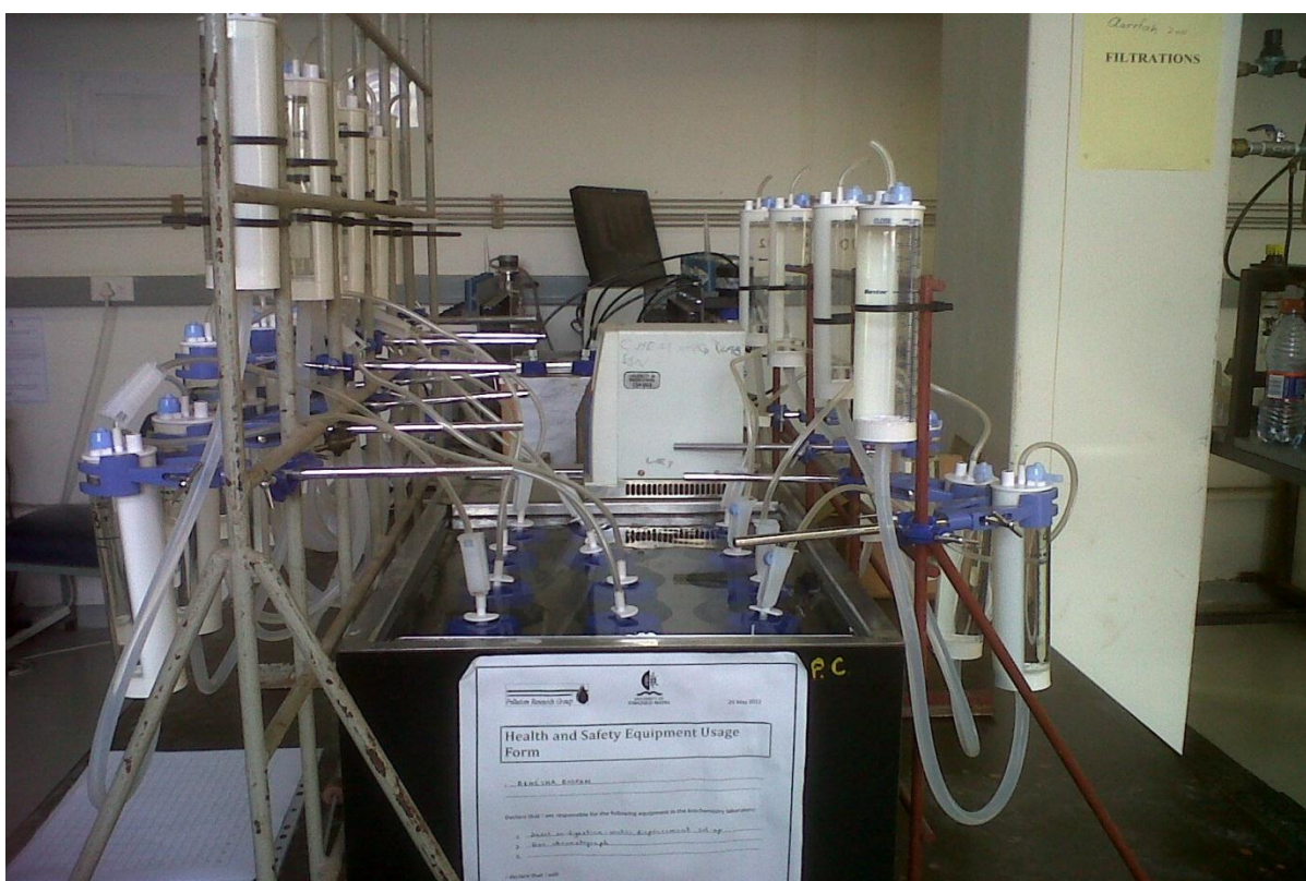
Figure 4.3: Photograph showing the attachment of the serum bottles in the water bath to the gas collection droppers
