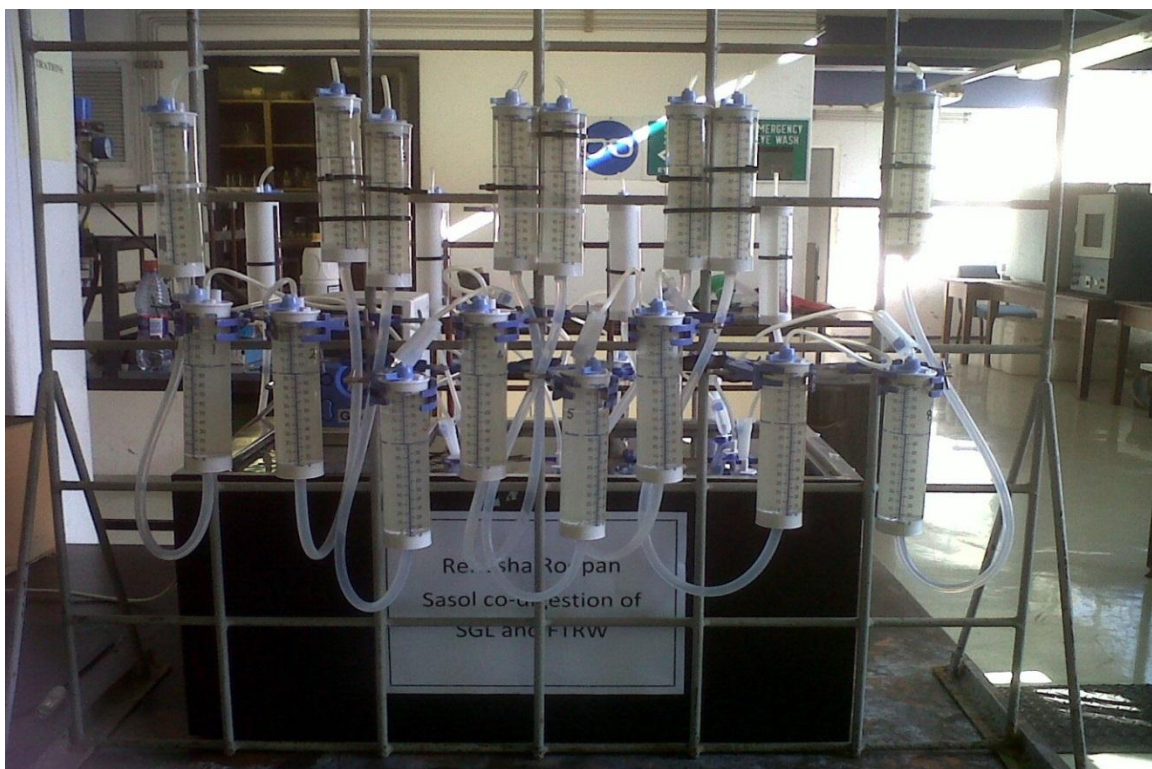
Figure 4.2: Photograph of the arrangement of the droppers with the bottom droppers being the gas collection droppers and the droppers above being the overflow chambers
