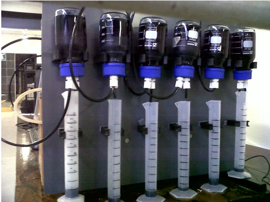
Figure 4.15: Photograph of the arrangement of the inverted bottles, filled with sodium hydroxide solution, above the plastic cylinders
