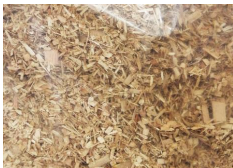
Figure 3-1: Photo of pin chips before milling into sawdust.
