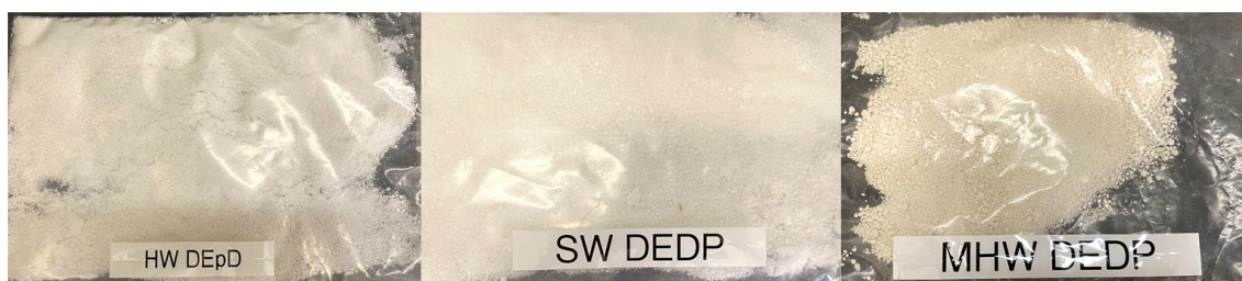
Figure 4-10: Air-dried, bleached, and blended grade of pulp.
