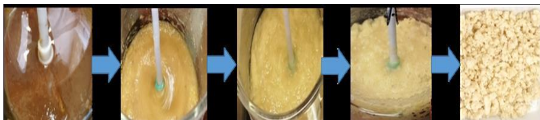
Figure 4-3: Transition of sawdust to pulp during benchtop delignification process using low temperatures between 60-70°C (Balkissoon et al., 2021).
