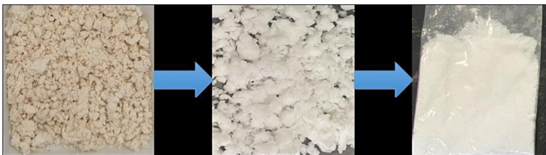
Figure 4-6: Transition of unbleached sawdust pulp, to bleached pulp and finally MCC following acid hydrolysis and spray drying.
