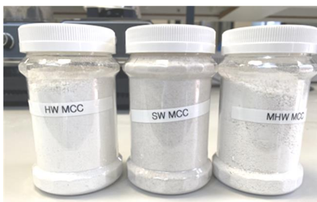
Figure 4-11: Prepared MCC variants following acid hydrolysis, air drying, and blending.
