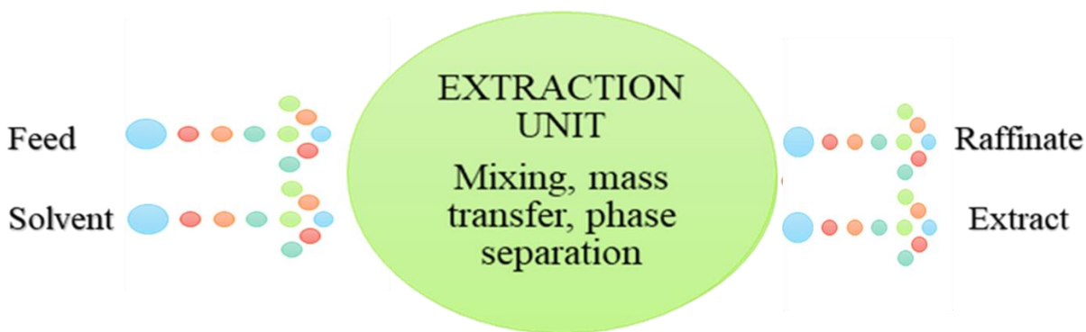
Figure 1.3: Illustration of the various elements in a liquid – liquid extraction system
