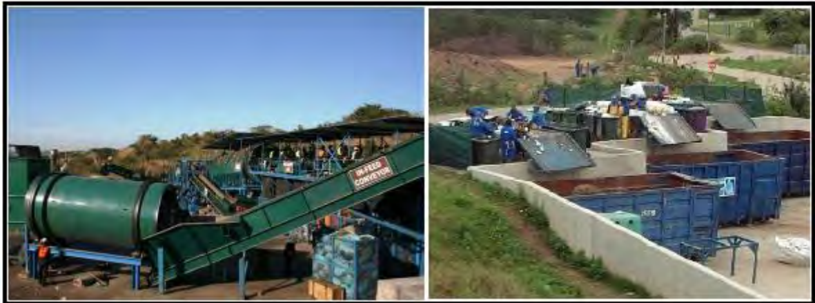
Figure 6.5 – Mechanical pre-treatment and pre-sorting line and initial sampling phase (Source: Re-ethical Environmental Re-engineering, 2009)
