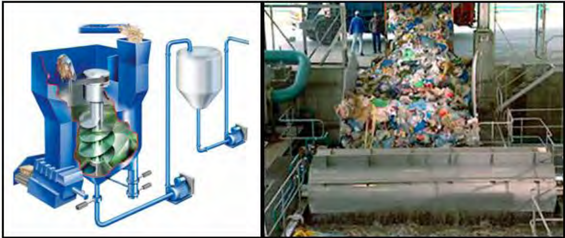
Figure 3.2 – Elements of pre-treatment: BTA hydro-pulper and Arrow Bio separation Tanks (Source: Arrow Bio, 2010; BTA Technology, 2010 and Biogen Greenfinch, 2009)
