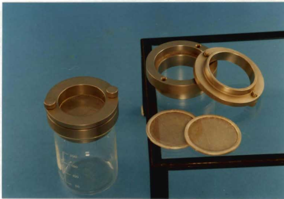
FIGURE A.3 Screen used for homogenization of liver tissue (Section A.3).
