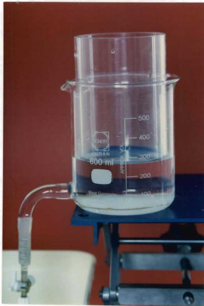
FIGURE C.2 Close-up of first-stage concentrator.
