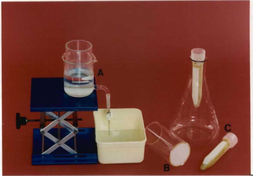
FIGURE C.1 Equipment used for concentration of cercarial suspensions: (A) First-stage concentrator; (B) Inner tube of first-stage concentrator; (C) Second-stage concentrator.
