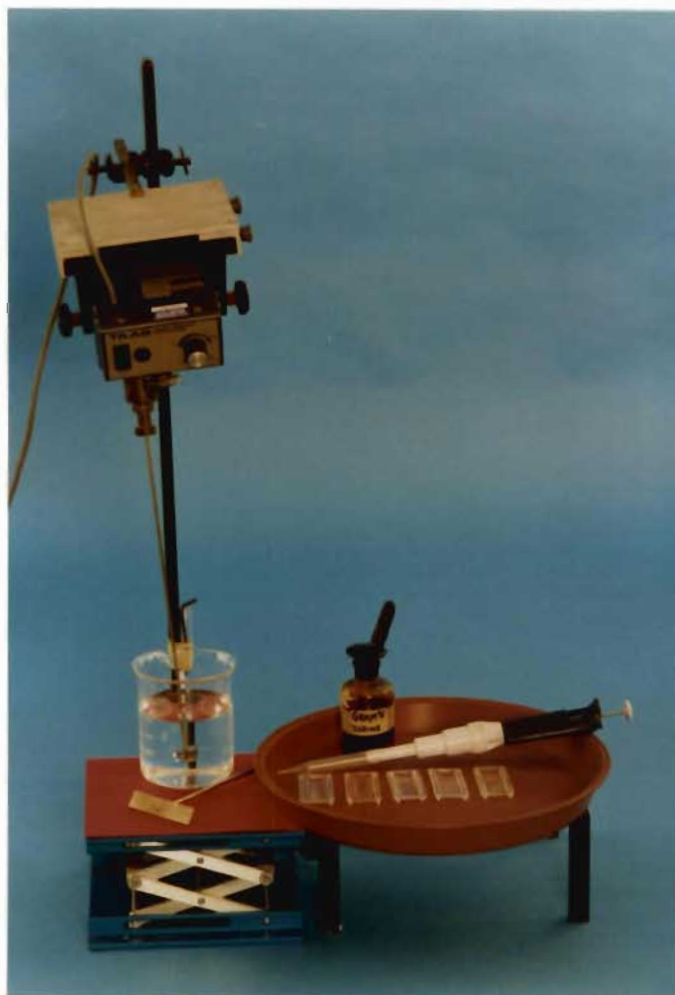
FIGURE A.5 Filtration of cercarial suspension to remove snail faeces.
