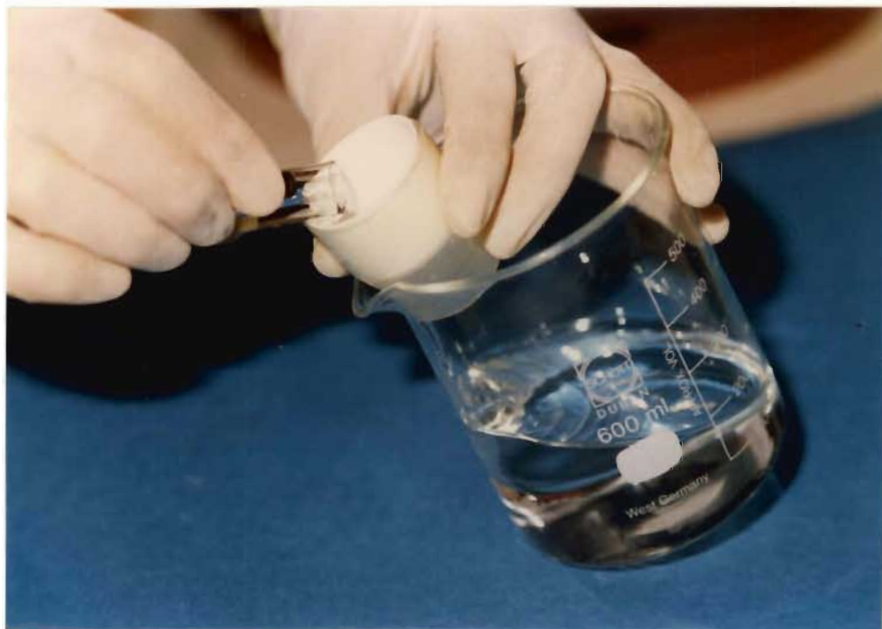
FIGURE A.5 Filtration of cercarial suspension to remove snail faeces.
