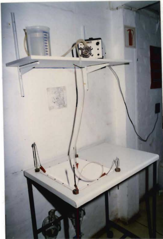
FIGURE 6.1 Apparatus used for recovery of schistosome worms from rats and guinea pigs. Tray dimensions (length x width x vertical depth) are 350 x 300 x 150mm.
