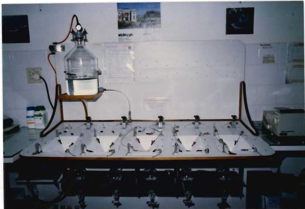
FIGURE 2.2 Perfusion apparatus used for the recovery of adult schistosome worms from mice and Mastomys coucha . This apparatus differs slightly from that described by Jackson et al (1982) in that worms are harvested under gravity rather than by suction. Tray dimensions (length x width x vertical depth) are 270 x 160 x 75mm.
