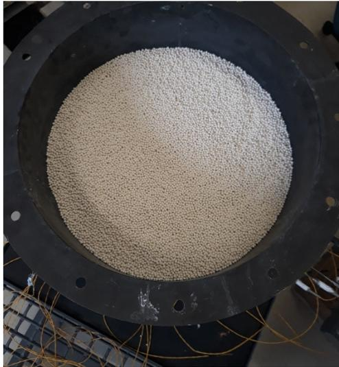
**Figure A-13: zeolite packed in reactor bed**
