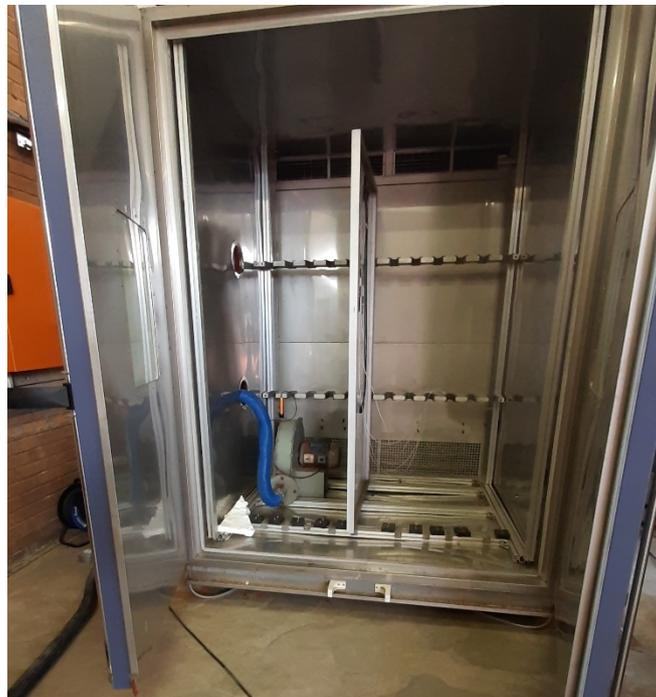
**Figure 5-26: Blower Placed in Humidity Chamber**
