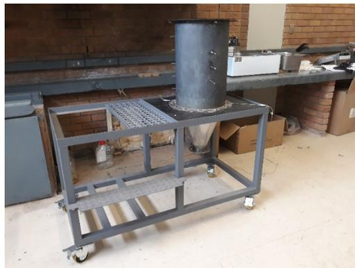
**Figure A-12: Reactor and Bottom Cone bolted together**
