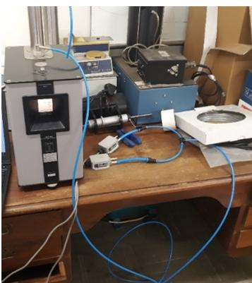
**Figure A-10: Pressure transducers connected to Betz manometer**
