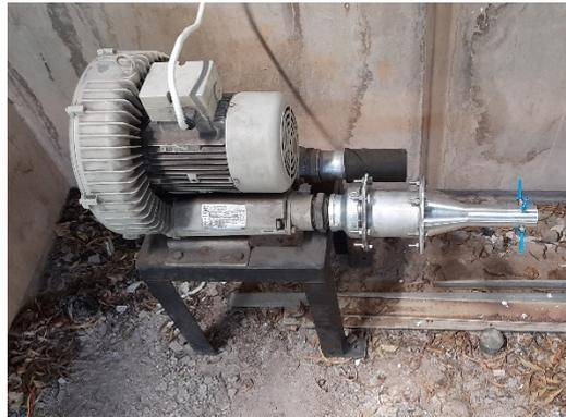
**Figure A-3: Centrifugal Blower with Conical Inlet Attached**
