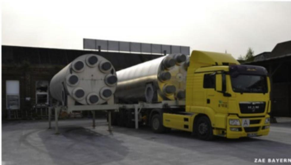
Figure 2-12: Mobile Sorption reactors [31]
