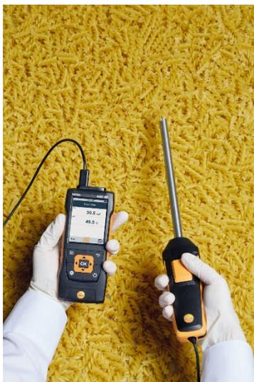
**Figure A-9: Testo humidity sensor and measurement device**
