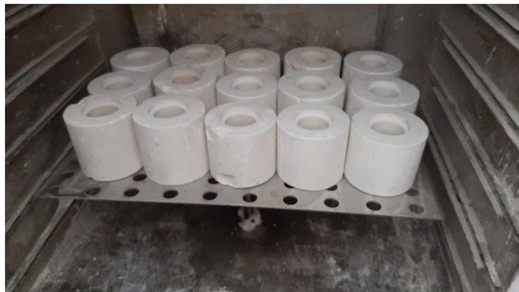
**Figure 5-20: Ceramic Moulds in Kiln**
