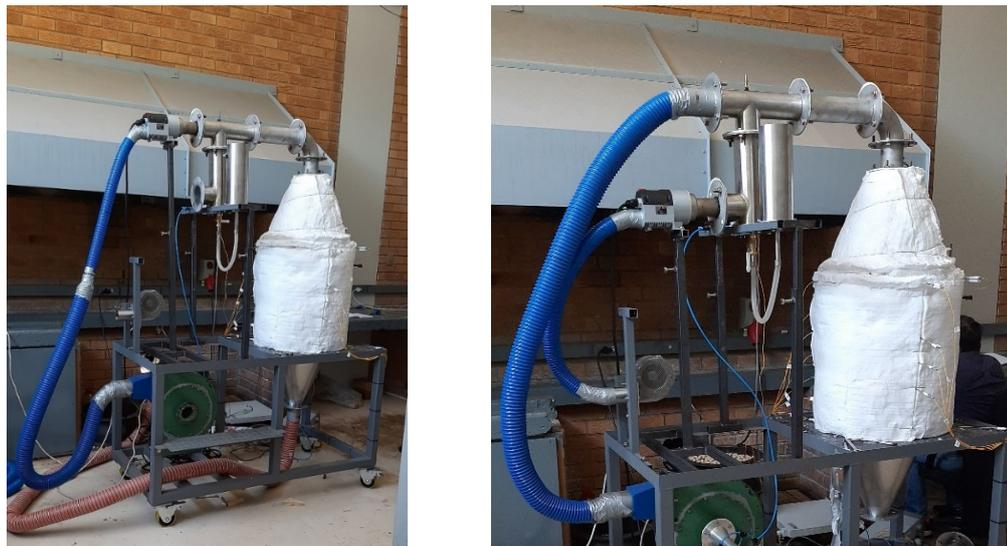
**Figure 3-4: Full Assembly showing charging (left) and discharging (right) configuration**
