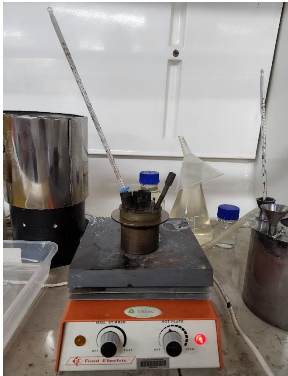
Figure E-2: Adapted Flash Point Property Set-Up.
