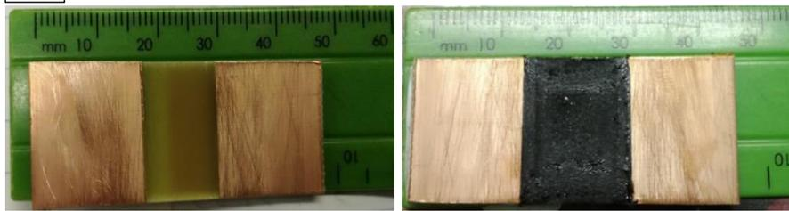
**Figure 4.30. The empty copper plate and the copper plate with ratio 1:1 PPy@NFC in PVA for dialysis-free Whatman filter paper.**
