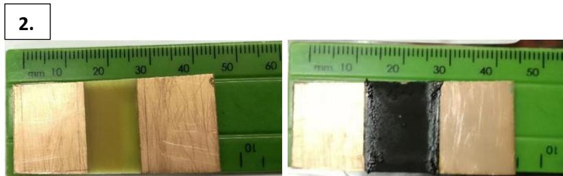
**Figure 4.28. The empty copper plate and the copper plate with ratio 1:1 PPy@NFC in PVA for dialysis-free hardwood pulp.**
