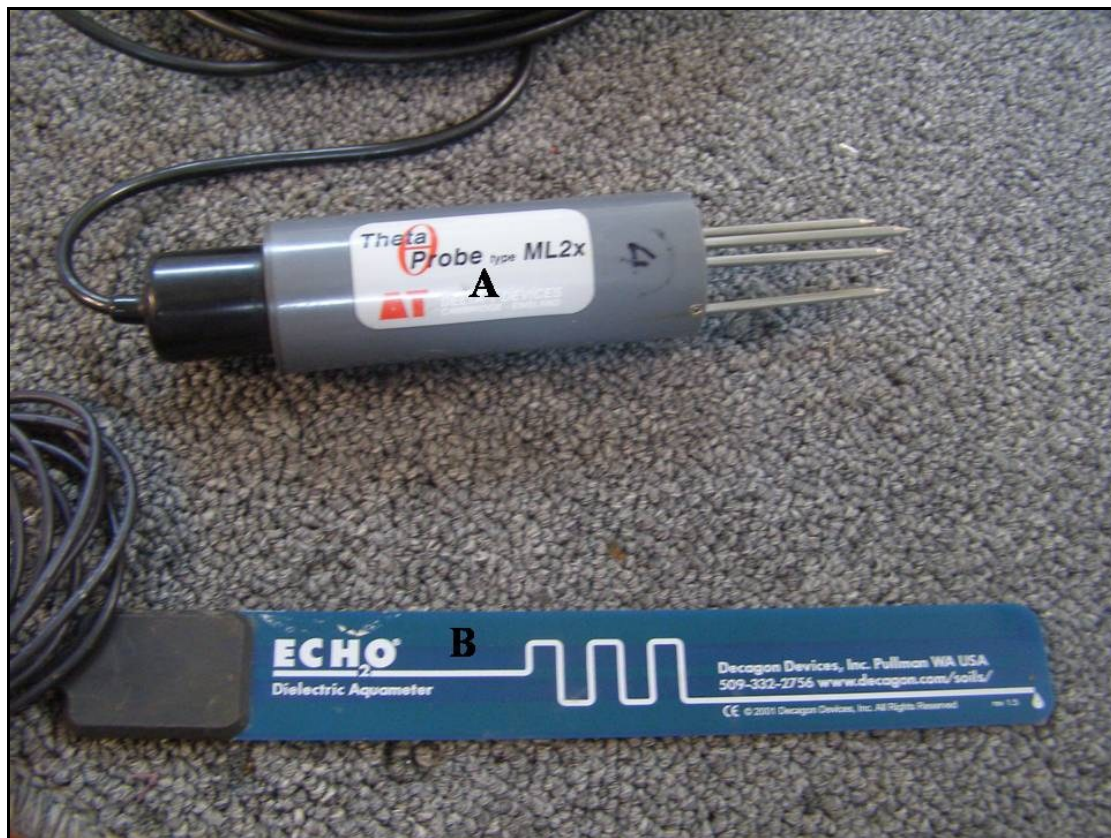
Fig. 3.2 ThetaProbe (A) and ECH 2 O Dielectric Aquameter (B) used for measuring soil water content.
