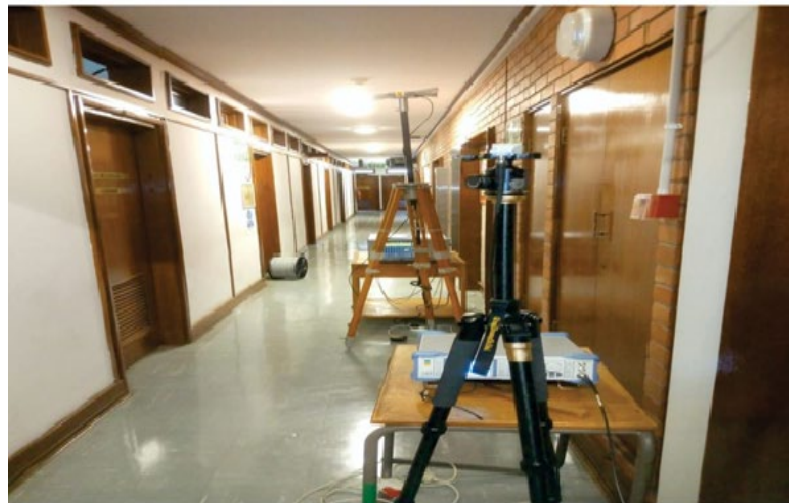
Figure 6.5. The Tx and Rx configuration in the indoor passage
