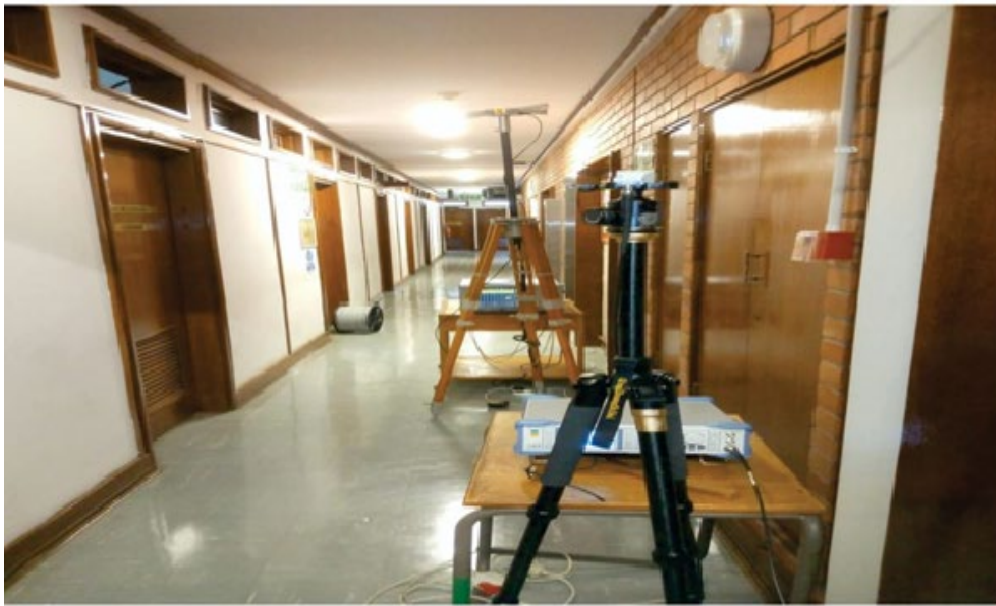
Figure 4.6. The setup of the Tx and the Rx in the indoor corridor environment.
