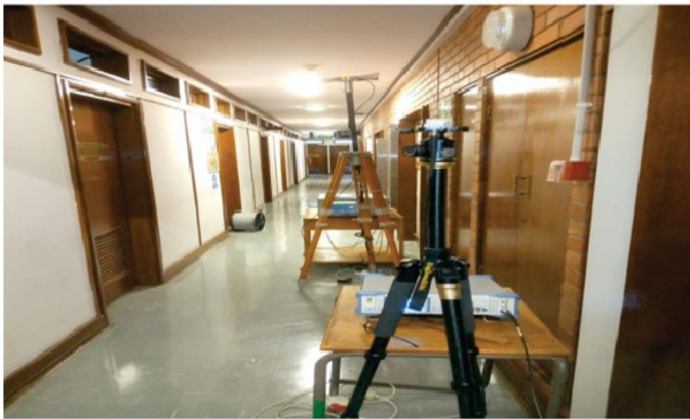
Figure 3.6. The setup of the transmitter and the receiver in the indoor corridor environment.
