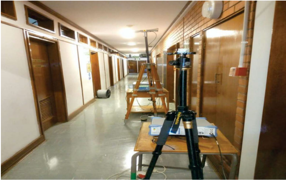
Figure 5.5. The configuration of the Tx and Rx in the indoor passage
