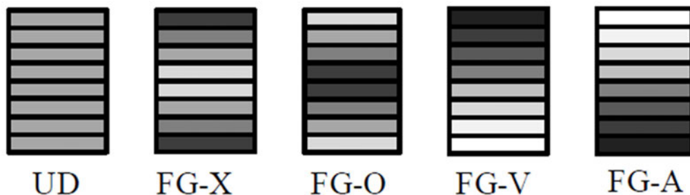
Figure 1.2: Functionally graded distribution patterns showing differing graphene content in the layers [9]
