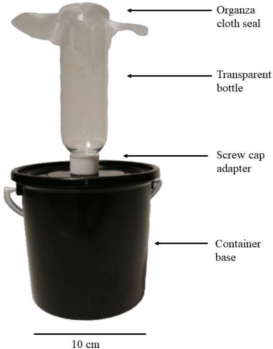
Fig. C1 Design of farm trial containers. Containers used were 12 cm tall × 10.5 cm wide. A 3 cm hole was drilled into each container lid and an inverted clear plastic bottle screw cap was attached and replaces. Plastic bottles were 14 cm tall × 4.5 cm wide and transparent to view fly emergence. The base of the bottles were removed and a piece of organza cloth was attached to allow for aeration and as a barrier preventing the entry or release of flies or larvae.
