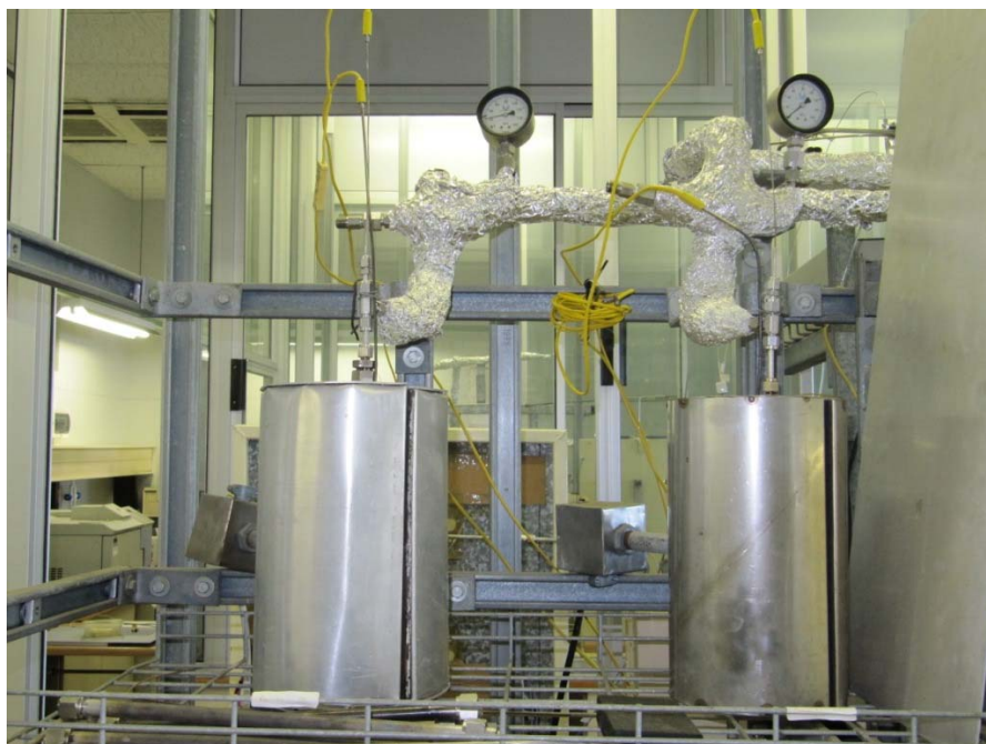
Figure A1.7 Reactors, pressure gauges and housing
