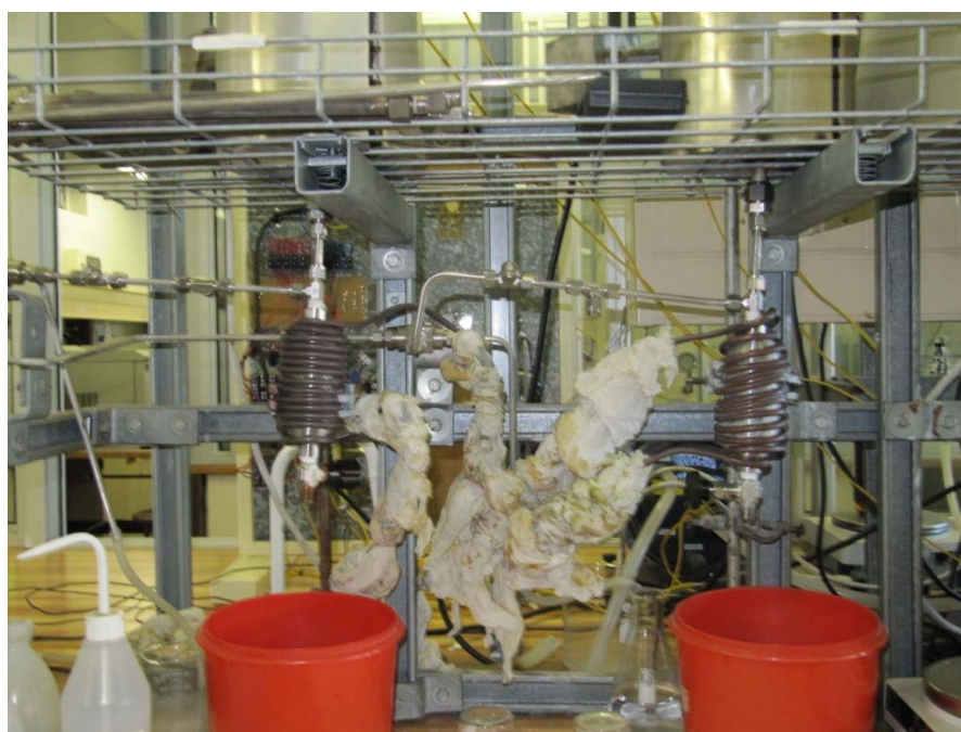
Figure A1.6 Catchpots for product streams
