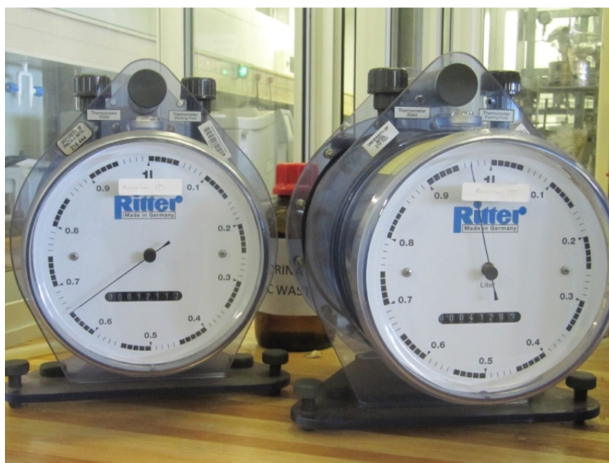
Figure A1.8 Ritter Wetgas flowmeters for off gas streams
