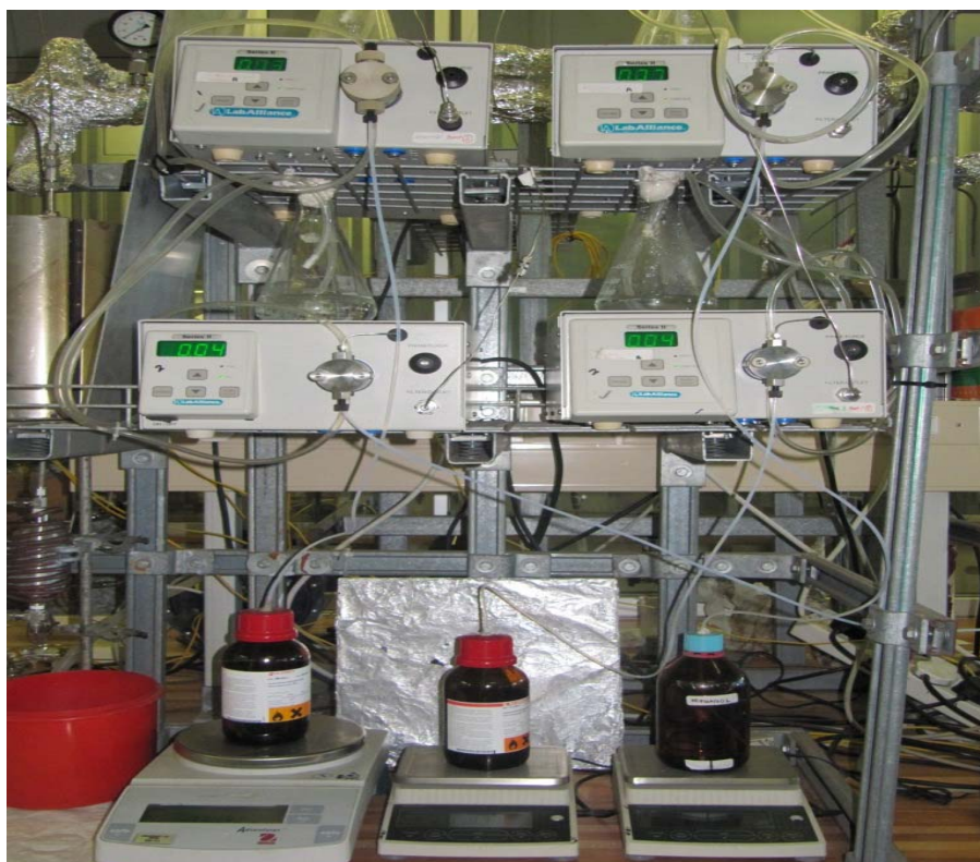
Figure A1.4 HPLC feed pumps and weighing balances
