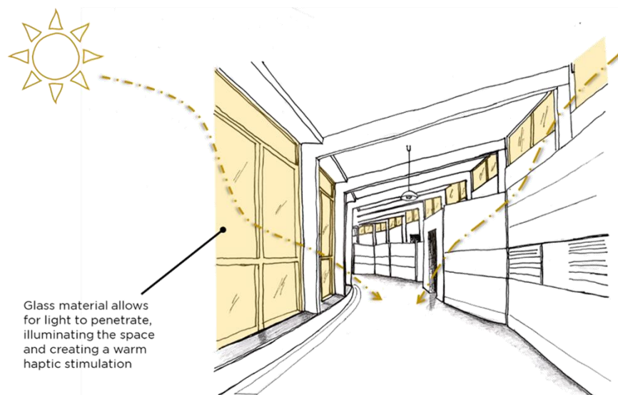
Figure 5.9 The usage of glass in the hallways allows for light to penetrate into the space and allow for spatial perception for visually impaired people through its contrasts of light and temperature. (Source: Architizer, n.d.; Adapted by Author, 2022)
