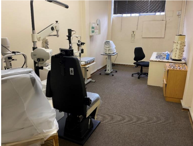
Figure 6.9 The clinic spaces utilize different flooring material to that found in the buildings haalways to signify a difference in the two spaces for the visually impaired. This material is then also used to code the clinic spaces throught the building. (Source: Author, 2022)
