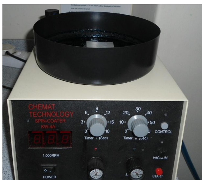
Figure 3.3: A photograph of Chemat spin coater (Model KW-4A) used in this study.
