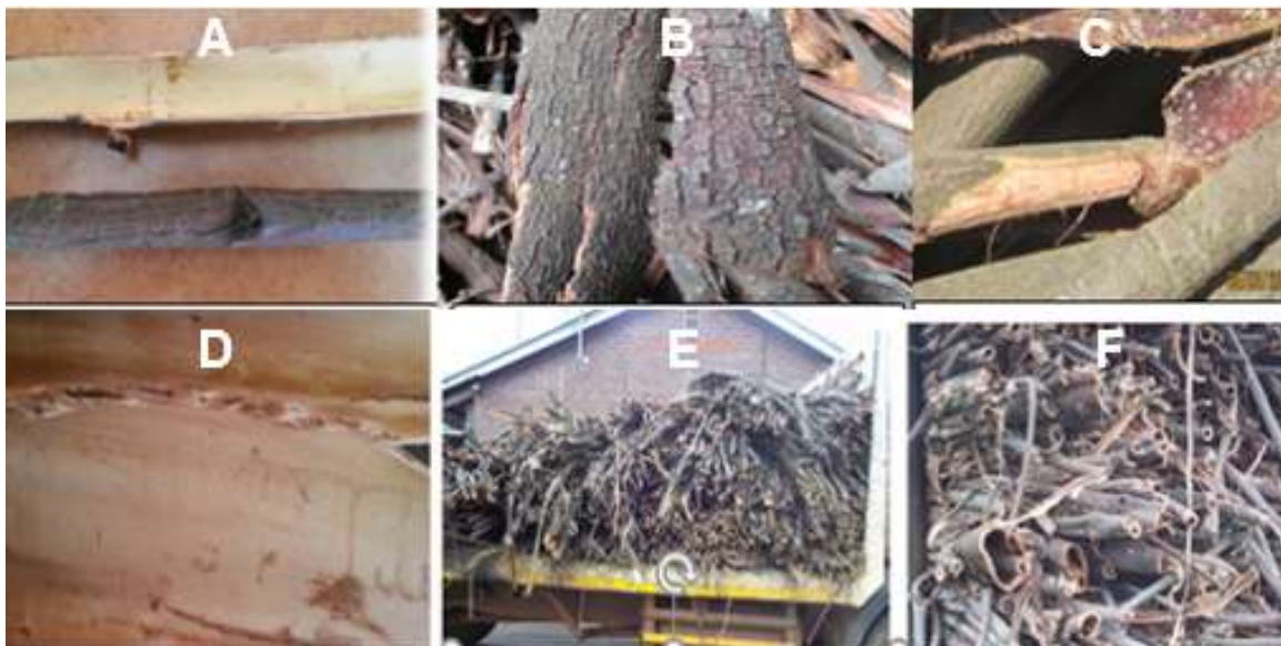
Figure 1.6 The several types of bark that are rejected due to inadequate quality as illustrated above (A) immature bark, (B) corky bark, (C) moldy bark, (D) green wattle, (E) poor presentation, and (F) dry bark (Source: Janse van Rensburg, 2022).
