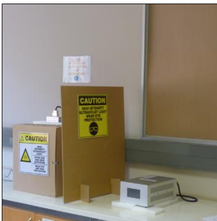
Figure 3.9: UVet UV LED array photochemical reactor system showing UV light protective reactor chamber, shield and window cover. These items were present to minimize the exposure of any non-participants to the UV light generated by the UV LED array source.
