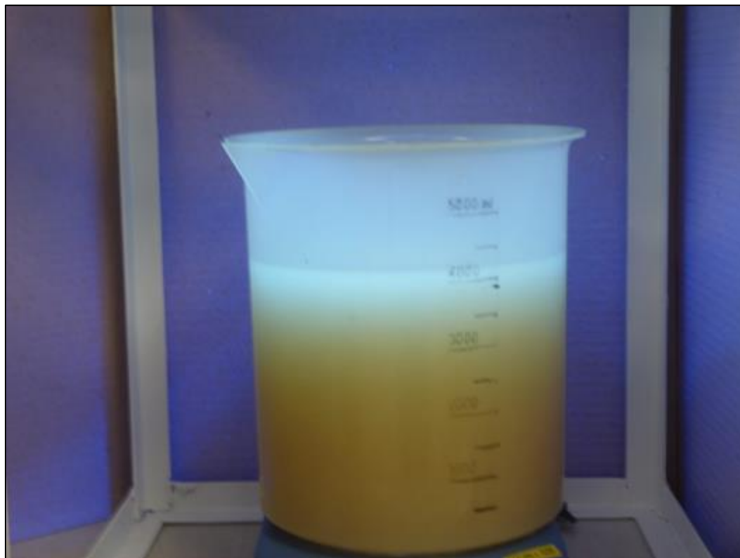
Figure 4.24: Visually observed extent of penetration given by scattered blue reflected light produced from UV irradiation using the UV LED array reactor.
