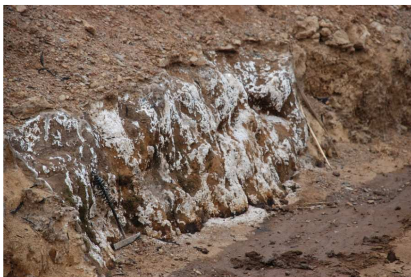
Plate 5.1: Calcrete exposed in a drain in Field D28 (East area). Hammer on the left is 30 cm long.
