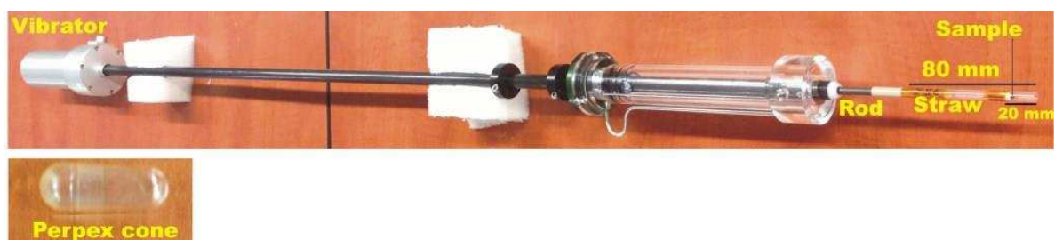
Figure 4.11: VTI VSM probe attached to a sample, Condensed Matter Physics Lab (WC), UKZN.
