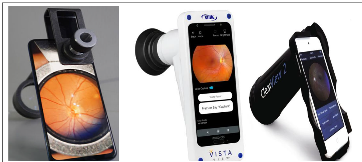
Figure 29: Mobile device equipped with retinal camera for portable wide field imaging Source: I-spot Vision (2022); Optibrand (2022); Volk (2023); Haddock et al. (2013)
