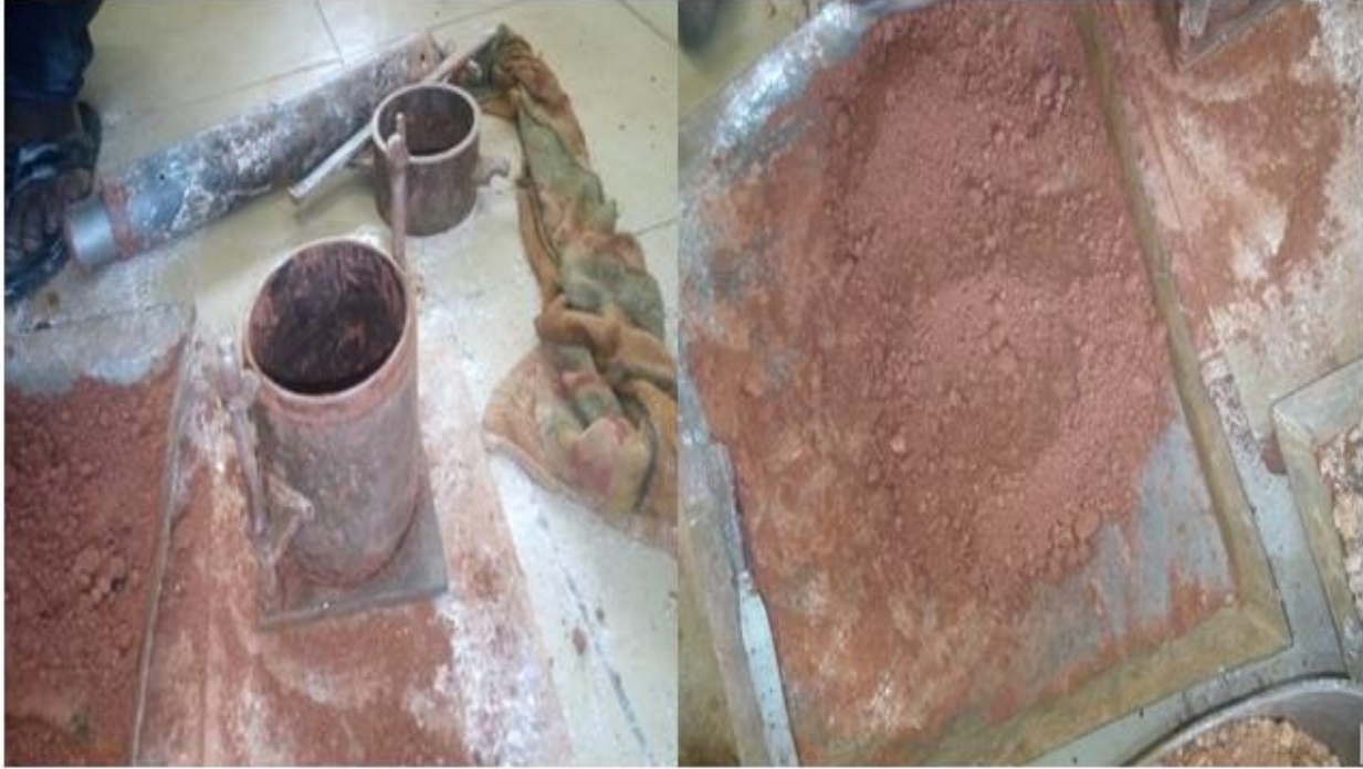
Figure 4.2. A compaction mould and the rammer with the lateritic soil to be compacted
