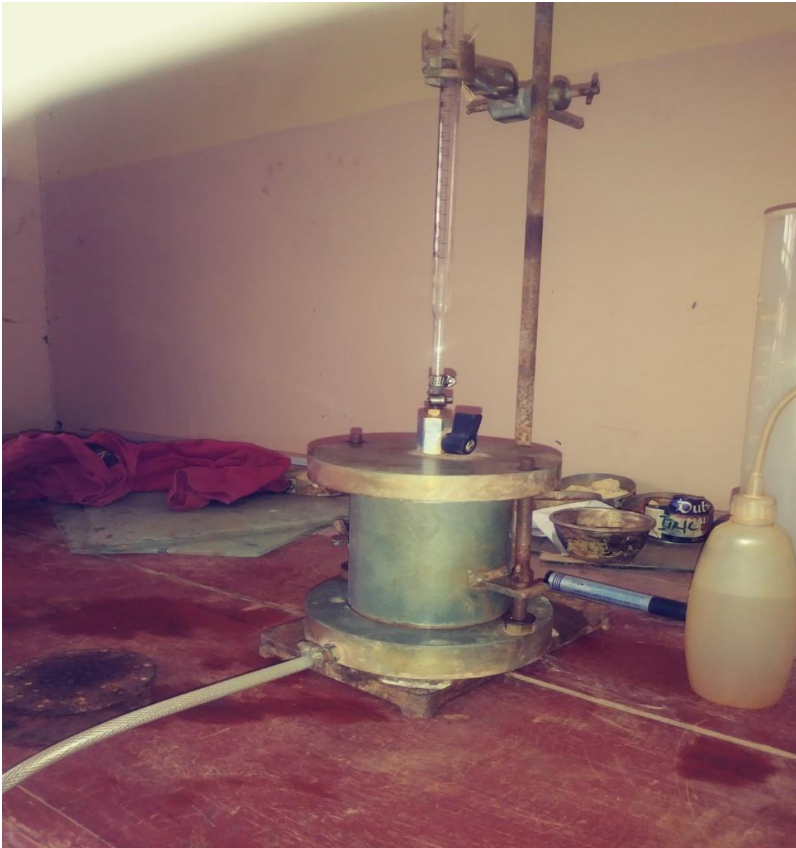
Figure 4.3. Typical setup of the falling head permeameter.
