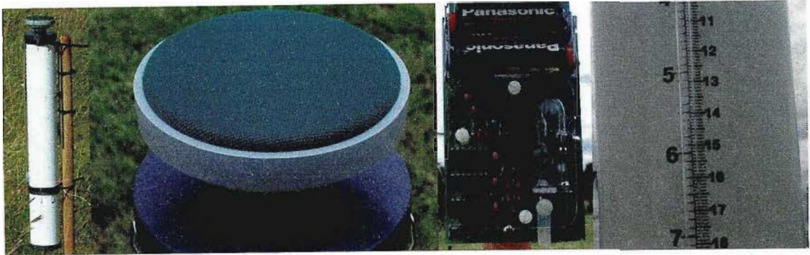
Fig. 5.2 Main parts of ET-gage atmometer (photograph, Savage 2001) from left to right: the complete unit, the ET-gage evaporation surface, the electronic board for model E and the glass sight tube. The diameter of the ET-gage evaporating sensor is 79 mm
