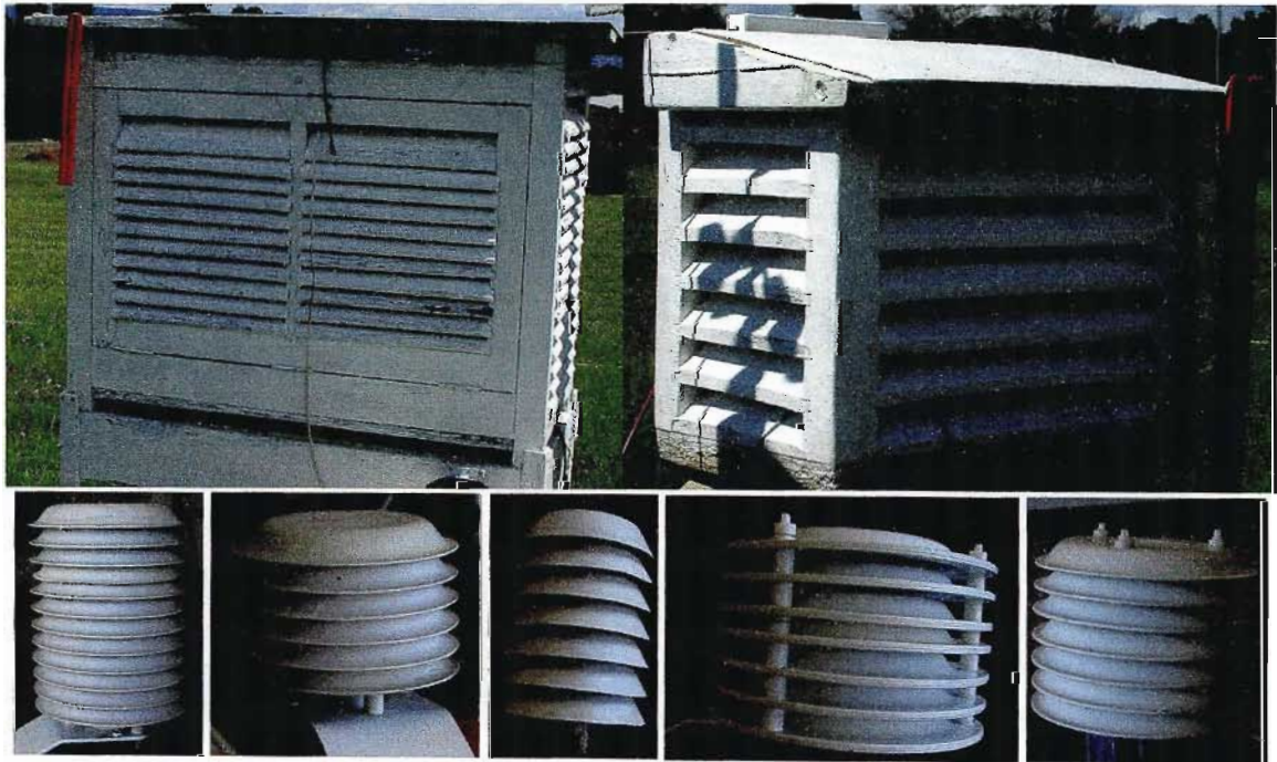
Fig. 5.4 Radiation shields from left to right: top standard Stevenson screen (910 mm × 720 mm × 460 mm), small Stevenson screen (300 mm × 200 mm × 270 mm) and bottom twelve-plate Gill radiation shield, six-plate Gill radiation shield, seven-metal plate home made radiation shield, seven-plate large size plastic home-made radiation shield, seven-plate small size plastic home made radiation shield
