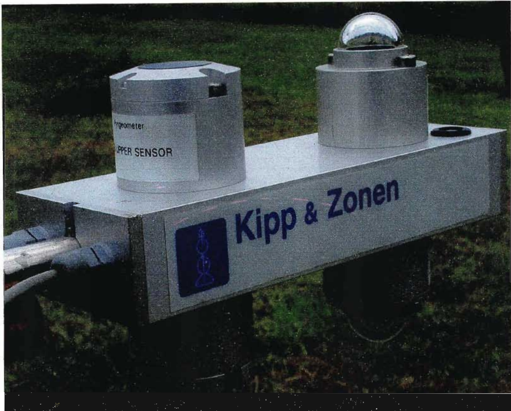
Fig. 5.1 Component net radiometer CNR1 for measuring the incident, reflected solar irradiance and incoming and outgoing long wave irradiance above a short grass surface (photograph, Savage 2001). The upper and lower CM3's are shown on the right
