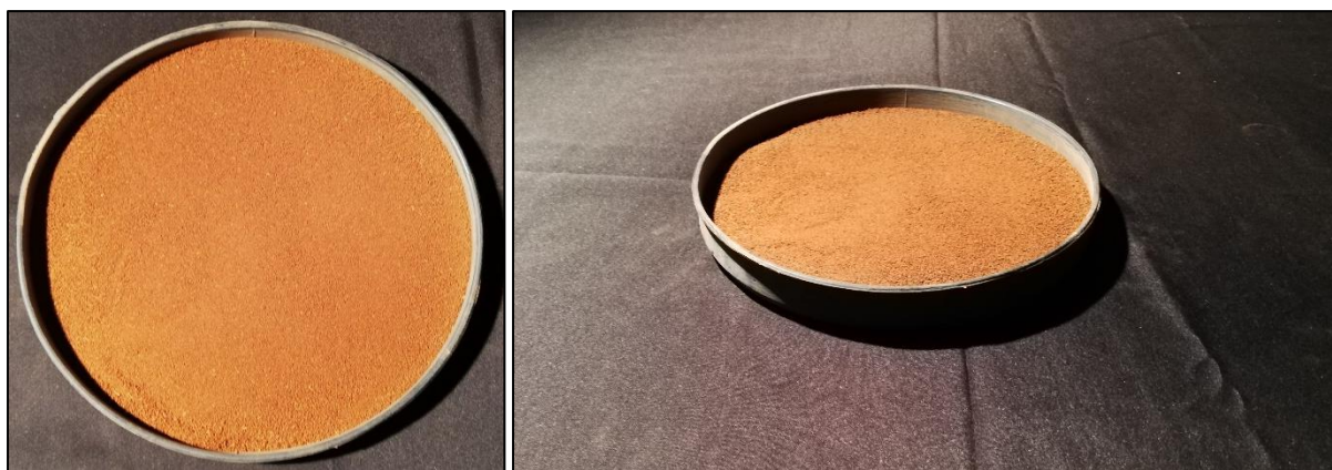
Figure 3.3: A soil sample that was levelled off to a smooth surface in a black plastic dish (Author, 2020)
