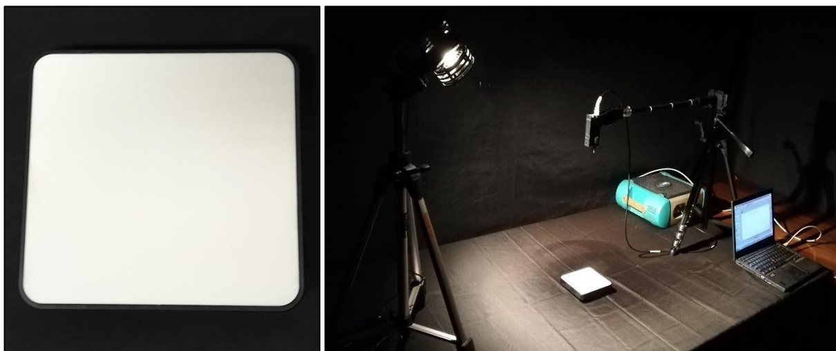
Figure 3.4: The white spectralon used to take a white reference measurement (Author, 2020)
