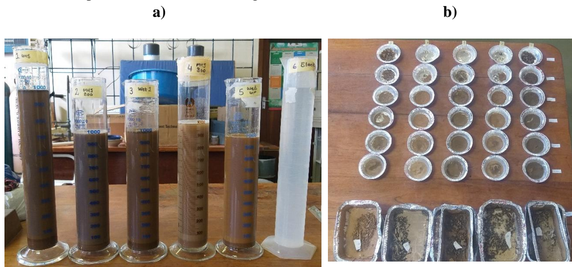
Figure 3.5 Laboratory setup and equipment for soil texture analysis: a) Samples prepared for analysis with hydrometer and b) sieved fractions of soil samples
