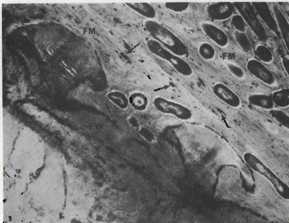
PLATE 3. Electron-opaque granules (arrows) embedded in a matrix of released fibrillar material (FM) both arising from bacterial action on the primary wall (PW) which has begun to swell and shred (broken arrow). The middle lamella (ML) is discontinuous. ( \times 20\ 500 .)
