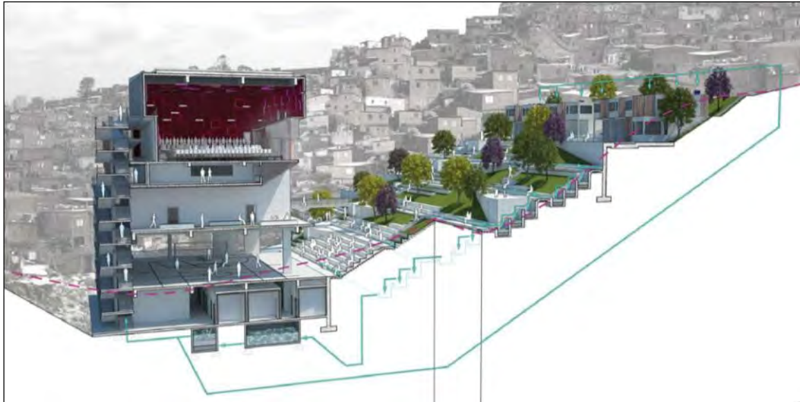
Figure 40: Section through site and intervention depicting housing at the top with terraces leading to main hub. Water storage tanks are indicated below the building. (Urban think Tank via (Holcim Awards, 2011))
