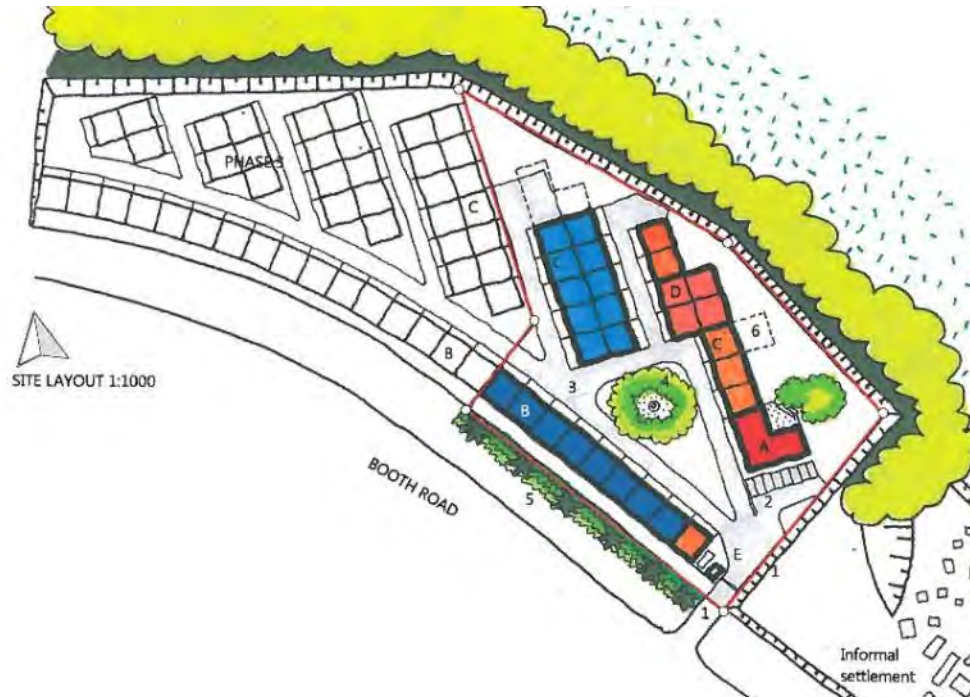
Figure 66: Site plan indicating current built design and future proposed phases. The bottom right (red) is the admin block which aids with surveillance of the entrance. The workshops are divided up according to size and use. The scheme is arranged around a central courtyard. (John Royal Architects)
