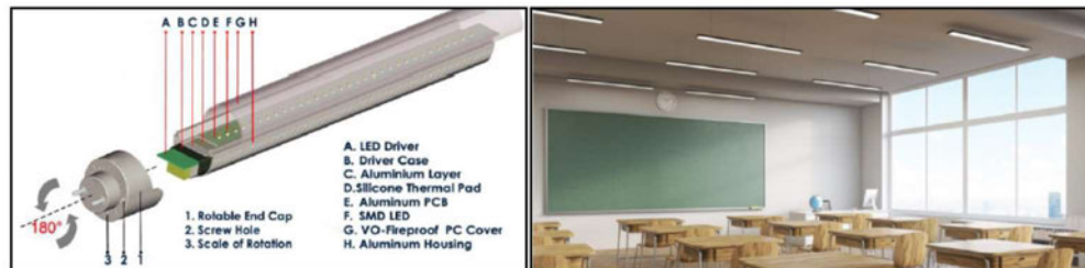
Figure 23: Left [9]: Typical components of LED Technology, Right [10] LED Lighting within an Environment
