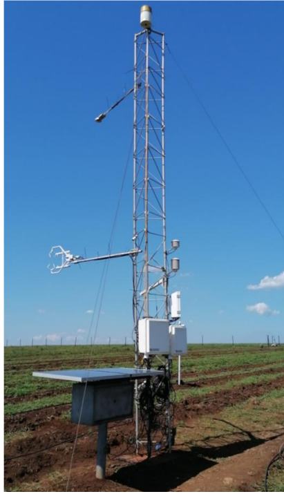
Plate 2.4: The 6 m tall eddy covariance system installed.
