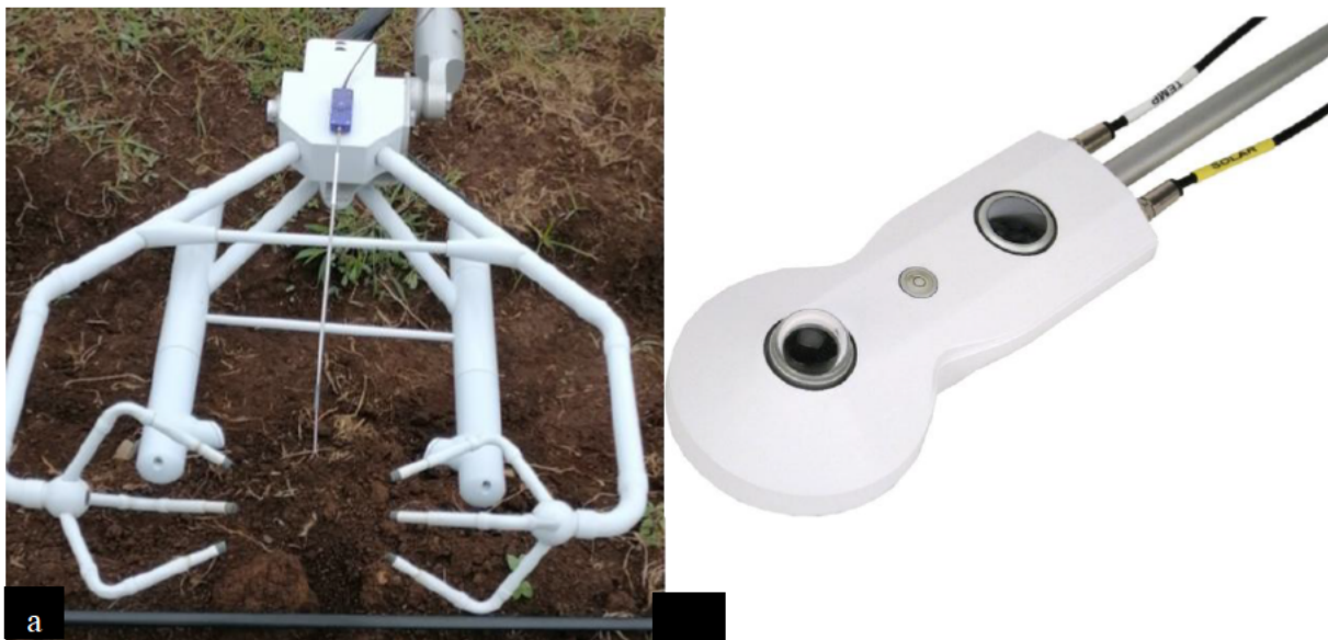
Plate 2.5: (a) Sensors including the CSAT3A, EC150 & FW1 attached together, (b) four component net radiometer.
