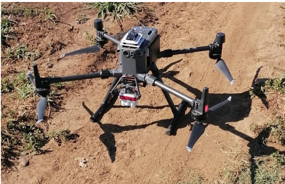
Plate 3.1: DJI Matrice 300 series drone with mounted MicaSense Altum camera, used for imagery acquisition over the growing season
