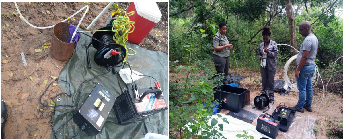
Figure 4-4 Pump used to purge the inactive (monitoring) boreholes
