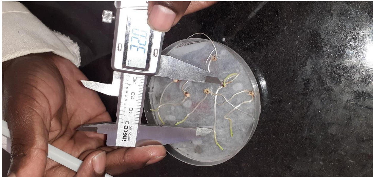
Figure 6. Taking of measurements for coleoptile length of sorghum seedlings using a digital Vernier Caliper as part of determination of thermotolerance in seedlings.
