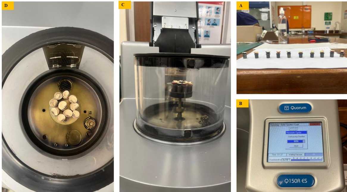
Figure 4.0.2: Preparing seed coat samples for scanning electron microscopy imaging. (A) seeds cryofractured in liquid nitrogen, split in half, and mounted on stubs using carbon adhesive tape; (B) gold coating of samples using a Quorum Q150R ES sputter coater; (C) sample stubs placed inside the sputter coater chamber during the coating process; (D) close-up view of gold-coated seeds mounted on stubs, ready for SEM imaging.
