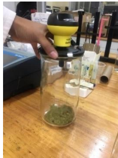
Figure 4.2 - 1: A setup for conducting biodegradability test
