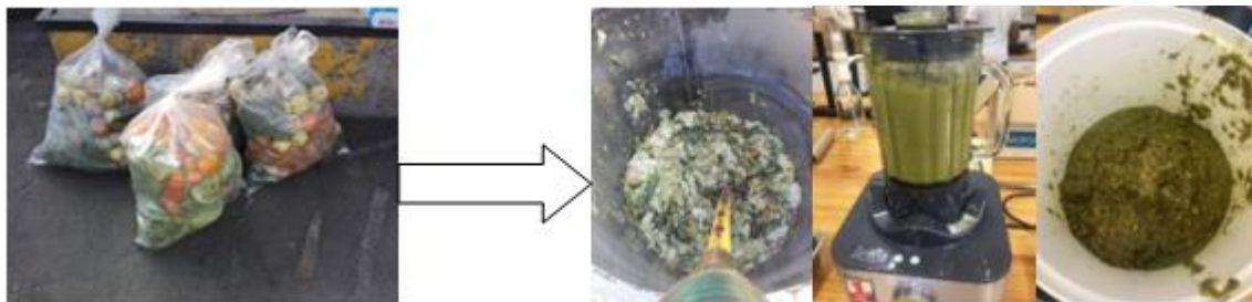
Figure 4.2 - 2: Collection and comminution of waste to the required size
