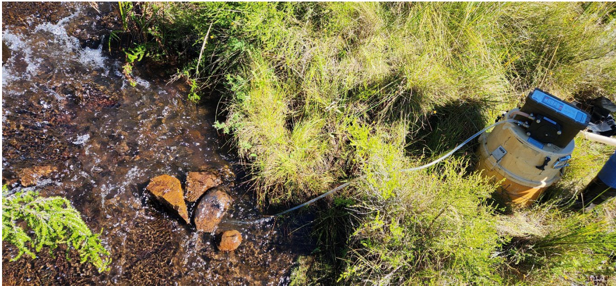
Figure 4-2: Event-based streamflow sampling setup below Wetland 2
