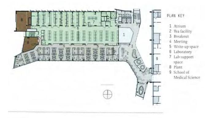
Fig. 4.1.8 Second Floor Plan (AA 2010)
