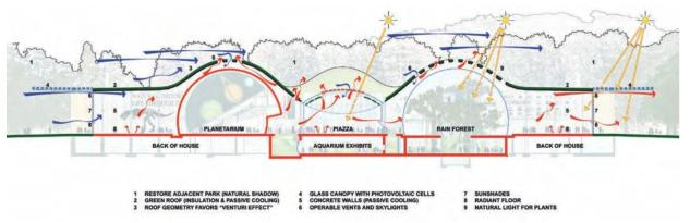
Fig. 4.3.8 Indoor air circulation (D + H 2011)
