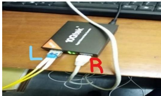
Figure 9: Electric to Fiber Optic Convert OR Fiber Optic to Electrical Converter
