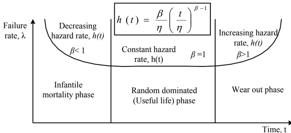
Figure 6-4: Weibull shape parameter and the bathtub curve
