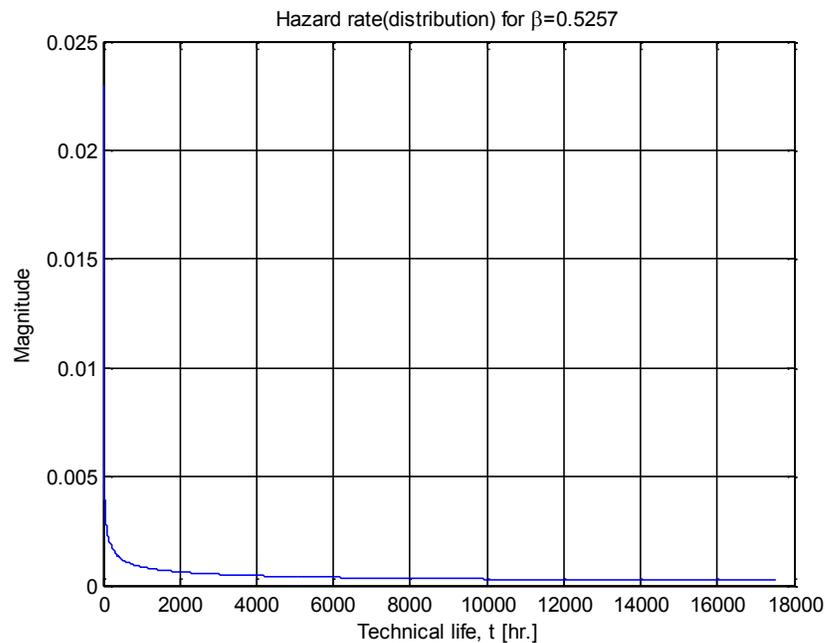
Figure 6-5: Hazard rates (distribution transformers)
