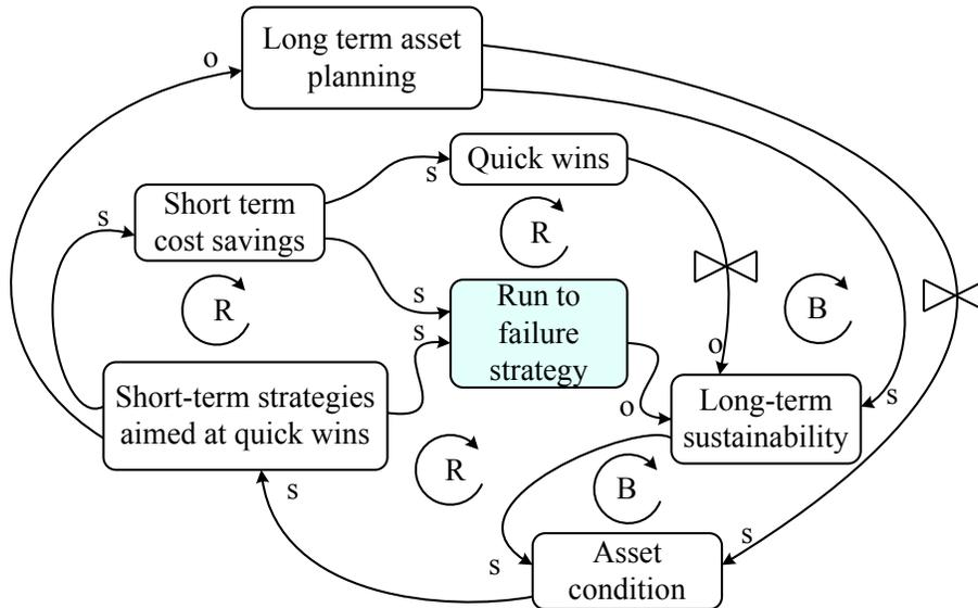
Figure 6-3: Systems view of run-to-failure strategy
