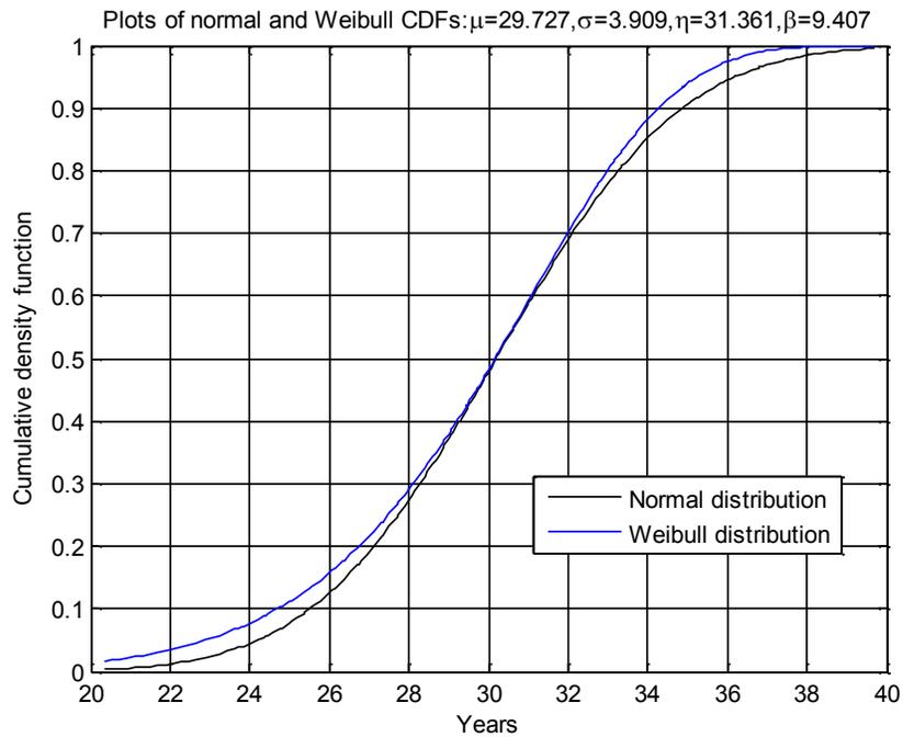
Figure 3-17: Comparison of Normal and Weibull CDFs for 500kV reactors
