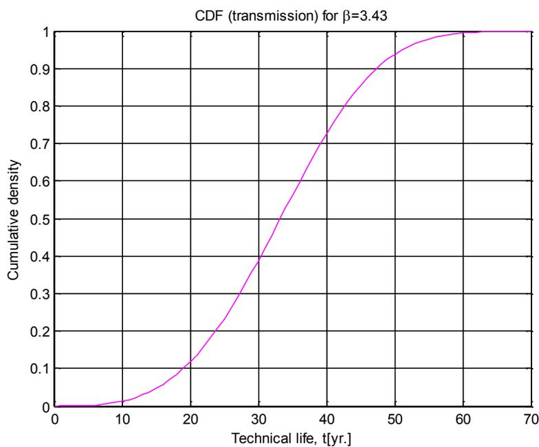
Figure 6-10: CDF (transmission transformers)
