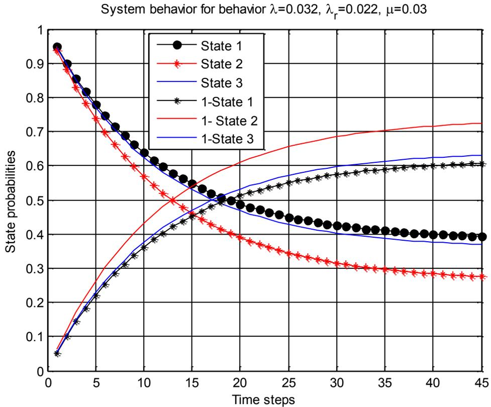
Figure 4-3: Generalized Markov transitional probabilities
