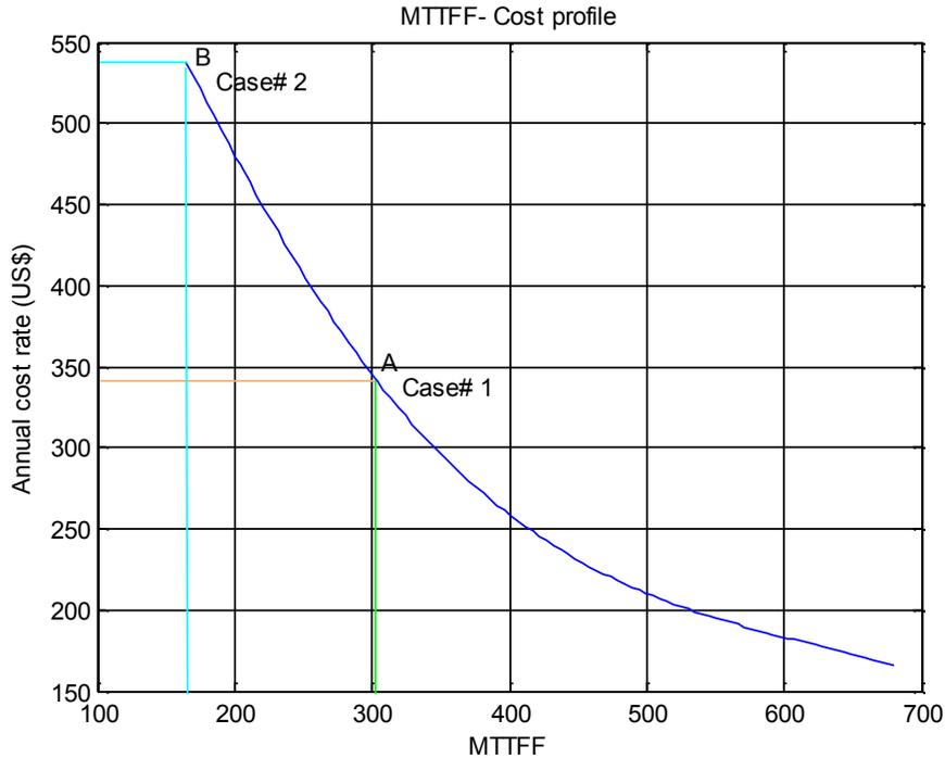
Figure 5-11: Variation of costs with the simulated values of the MTTFF
