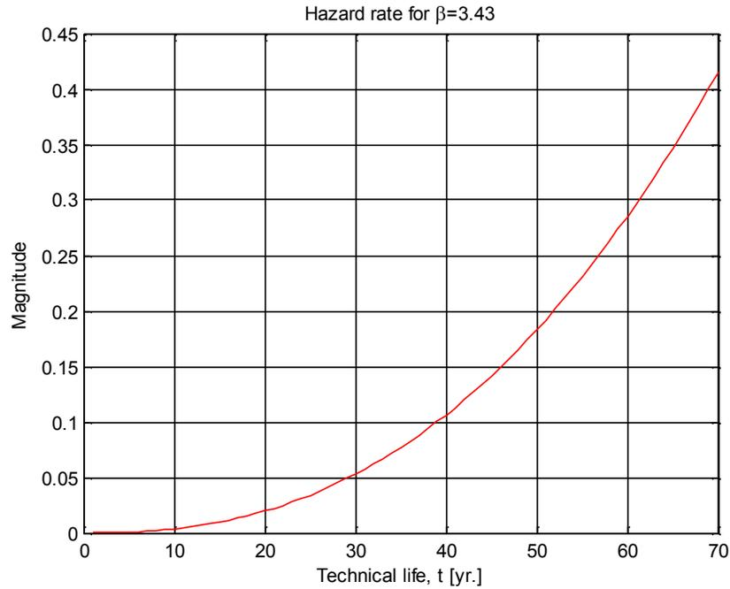
Figure 6-6: Hazard rates (transmission transformers)
