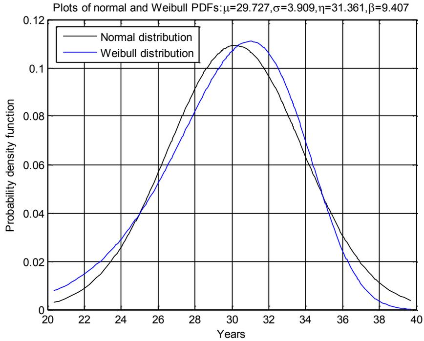
Figure 3-16: Comparison of Normal and Weibull PDFs for 500kV reactors
