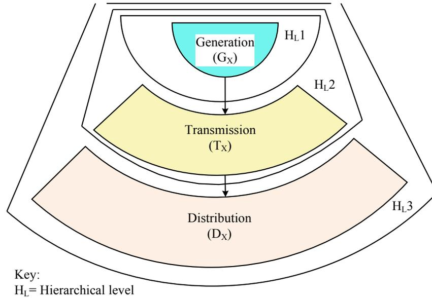
Figure 2-1: Power system functional (hierarchical) levels
