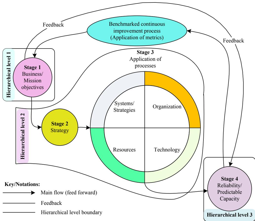
Figure 2-3: Hierarchical levels of AM systems
