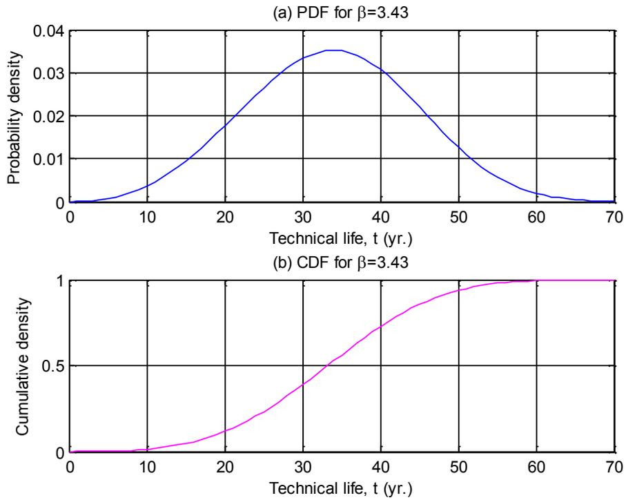
Figure 3-10: (a) PDF and (b) CDF based on the technical life
