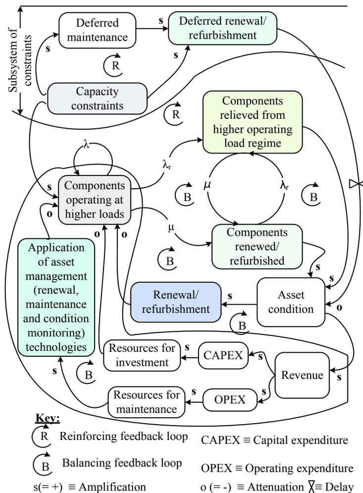
Figure 4-1: Power grid management system as a system of subsystems
