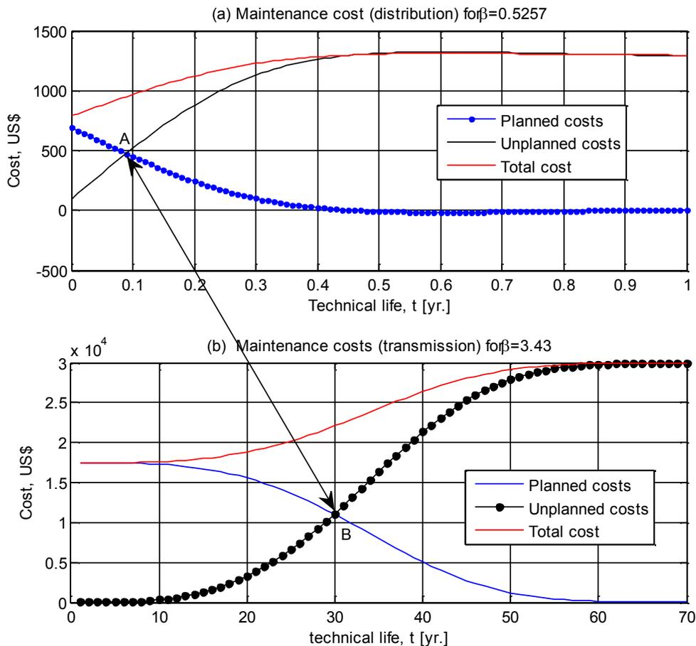
Figure 6-11: Comparison of costs: (a) distribution and (b) transmission transformers
