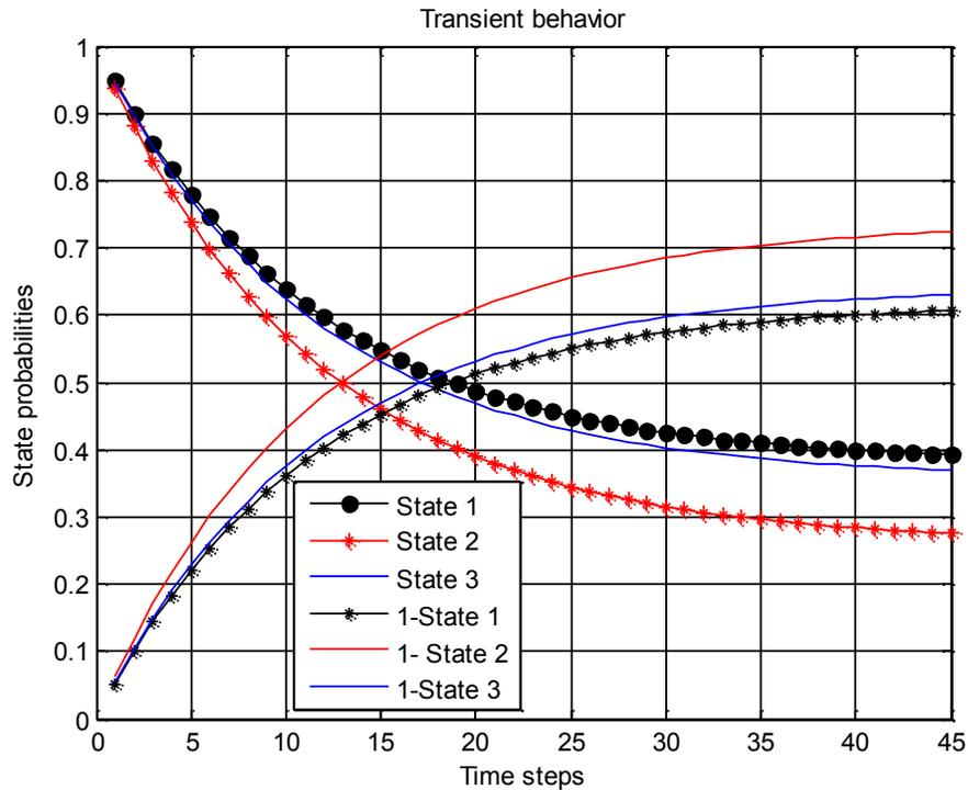
Figure 3-5: Transient behavior in the context of a generalized Markov process
