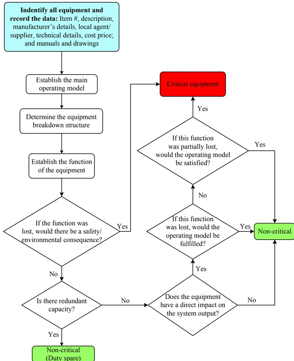
Figure 5-1: Equipment criticality determination (adapted from [10])
