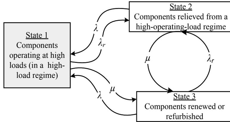
Figure 3-4: State-space transition in the context of a generalized Markov process
