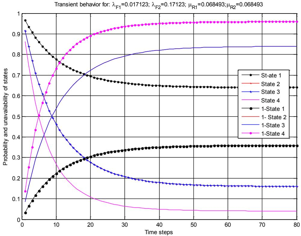
Figure 5-9: Transient probabilities for case #5
