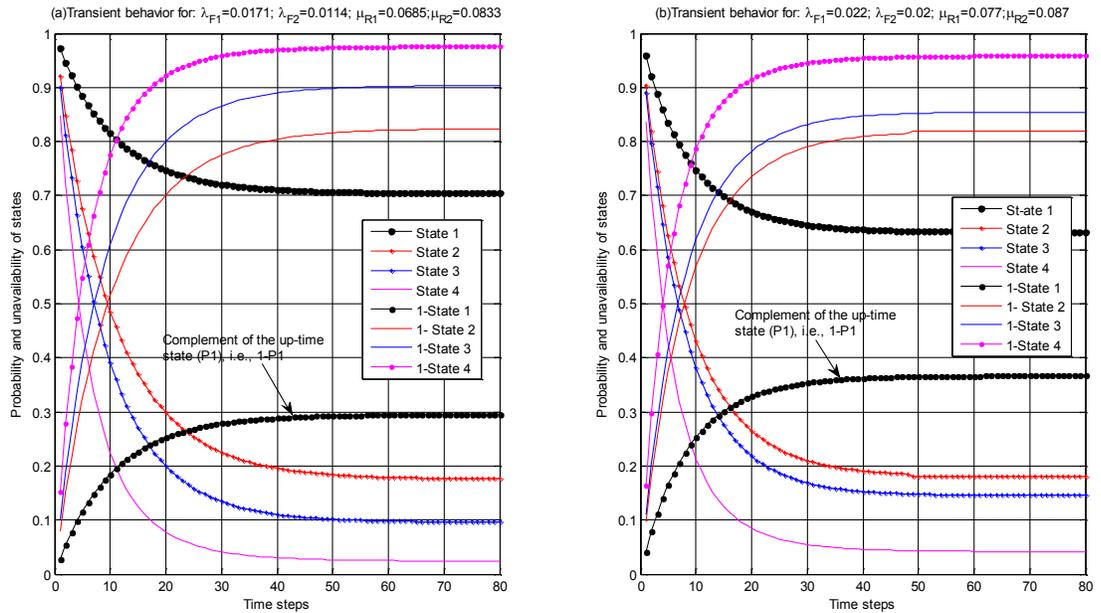
Figure 5-6: Transient probabilities for cases 1 and 2
